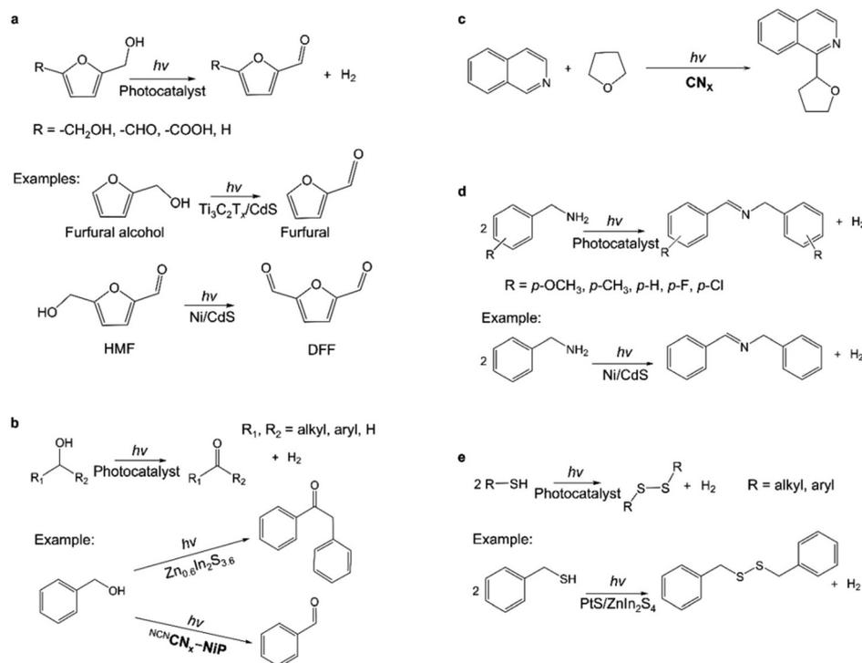
**Fig. 4** (a) Photocatalytic oxidation of biomass-derived intermediate compounds.<sup>52,54,56</sup> HMF: 5-hydroxymethylfurfural; DFF: 2,5-diformylfuran. (b) Photocatalytic oxidation of alcohols.<sup>57,58</sup> (c) Photocatalytic Minisci coupling.<sup>59</sup> (d) Photocatalytic C–N coupling reactions.<sup>56,60</sup> (e) Photocatalytic S–S coupling reactions.<sup>56,61</sup>
