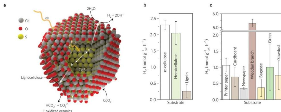
**Fig. 2** (a) Diagram of the photoreforming of lignocellulose to  $H_2$  on CdS/CdO<sub>x</sub>. (b and c) Photocatalytic production rates of  $H_2$  from  $\alpha$ -cellulose, hemicellulose and lignin (b), and raw and waste biomass substrates (c) using Co/CdS/CdO<sub>x</sub> quantum dots in 10 M KOH aqueous solution under simulated solar light (AM 1.5G, 100 mW cm<sup>-2</sup>). Reproduced with permission from ref. 24. Copyright 2017 Macmillan Publishers Limited, part of Springer Nature.
