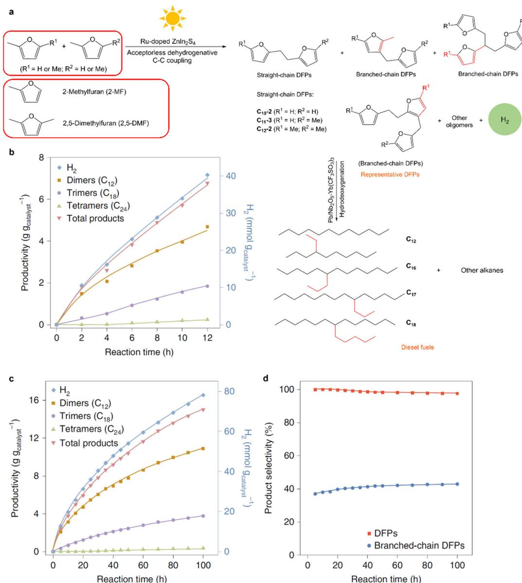
**Fig. 5** (a) Schematic representation of the photocatalytic transformation of 2,5-DMF/2-MF into diesel fuel. (b–d) Photocatalytic dehydrocoupling of 2,5-DMF as a substrate: standard experiment (b), catalyst lifetime evaluation (c), and selectivity to oxygenated DFPs and branched-chain DFPs (d). Reproduced with permission from ref. 68. Copyright 2019 Springer Nature Limited.
