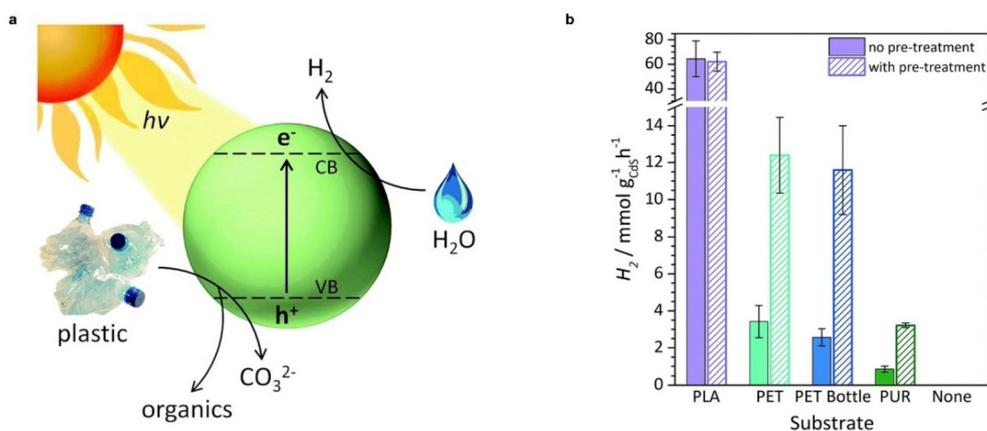
**Fig. 3** (a) Diagram of the photoreforming of plastic waste using a CdS/CdO<sub>x</sub> quantum dot photocatalyst. (b) Photoreforming of polymers to H<sub>2</sub> using CdS/CdO<sub>x</sub> quantum dots under simulated solar light (AM 1.5G, 100 mW cm<sup>-2</sup>). Reproduced with permission from ref. 37. Copyright 2018 The Royal Society of Chemistry.
