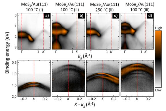
Fig. 4 Angle-resolved UP spectra of (a) MoS<sub>2</sub> (i) annealed at 100 °C, MoSe<sub>2</sub> (iii) annealed at (b) 100 °C and at (c) 250 °C as well as (d) MoSe<sub>2</sub> (iii) on Au(111) annealed at 100 °C. In the top parts, the band structures along  $\Gamma$ -K direction are shown. Below, detailed parts of the band structure acquired with the 2D detector around the K points are presented.
