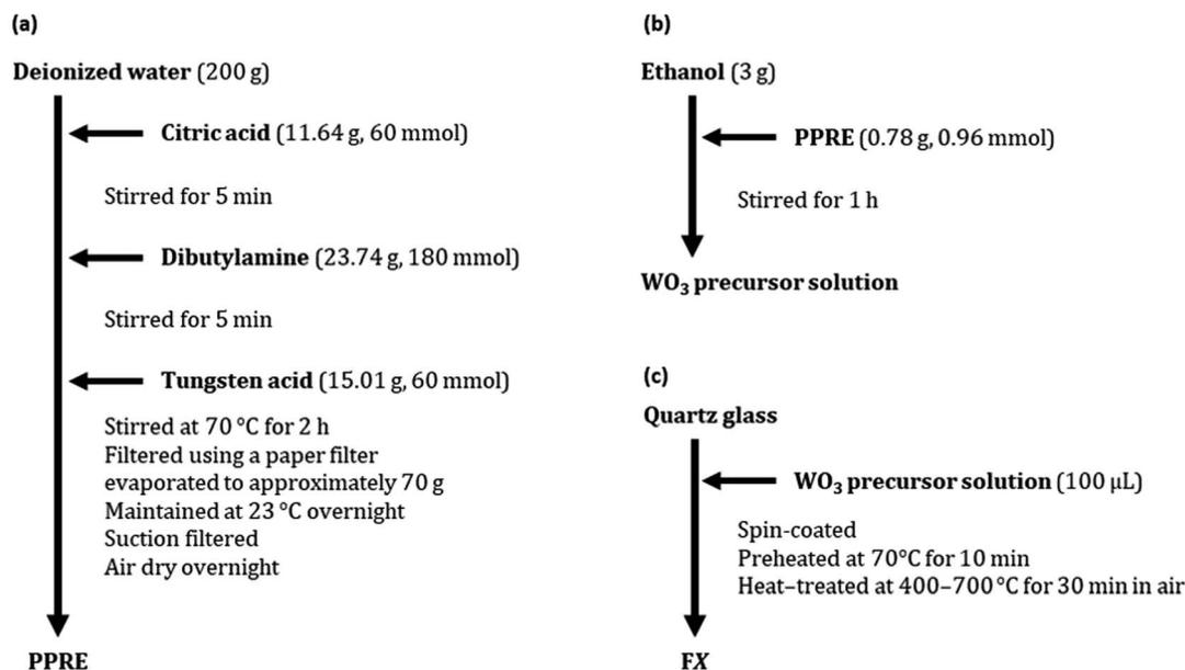
Fig. 1 The experimental routes for (a) the isolated PPRE and (b) the WO<sub>3</sub> precursor solution dissolving the powder and (c) the procedures for coating and heat treatment.
