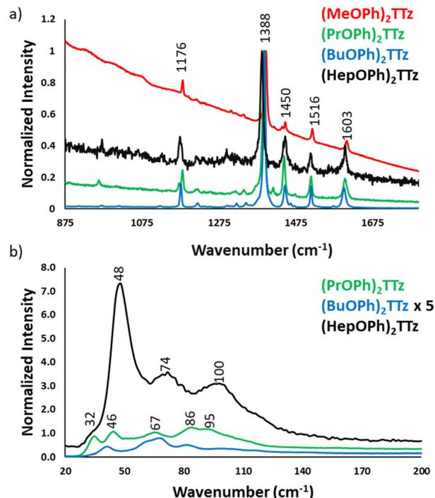
Fig. 7 Micro-Raman spectra of TTz crystals.
