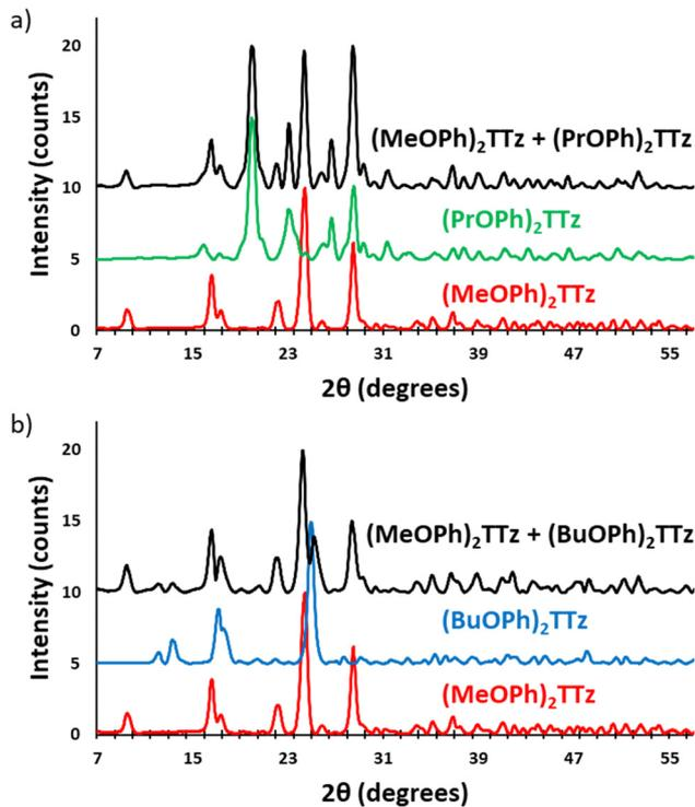
Fig. 9 Powder X-ray diffractograms of parent TTz crystals and their blends. (a) Set 1:  $(\text{MeOPh})_2\text{TTz}$ ,  $(\text{PrOPh})_2\text{TTz}$ , and  $(\text{MeOPh})_2\text{TTz} + (\text{PrOPh})_2\text{TTz}$  crystalline blend; (b) set 2:  $(\text{MeOPh})_2\text{TTz}$ ,  $(\text{BuOPh})_2\text{TTz}$ , and  $(\text{MeOPh})_2\text{TTz} + (\text{BuOPh})_2\text{TTz}$  crystalline blend.
