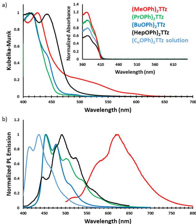
Fig. 5 Steady state photophysical characteristics of symmetrically substituted dialkoxyphenyl TTz crystals. (a) Absorption spectra of TTz crystals obtained *via* diffuse reflectance spectroscopy. Inset: UV-Vis absorption spectra of TTzs in solution state. (b) Photoluminescence spectra of TTz crystals and solution.
