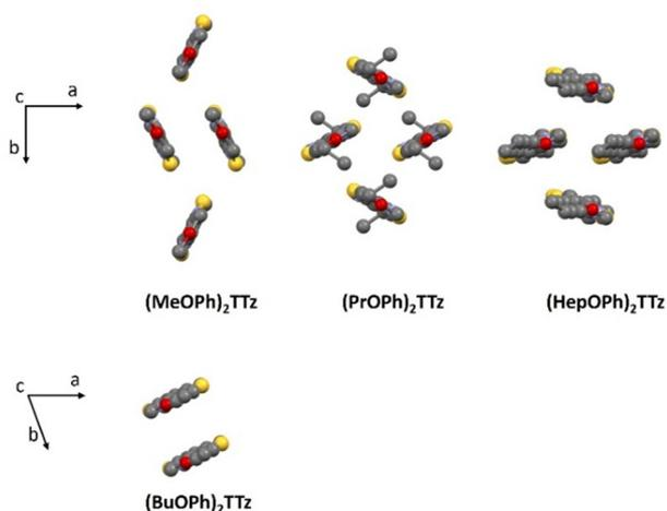
Fig. 2 Crystal packing diagram of (C<sub>n</sub>Oph)<sub>2</sub>TTz unit cell. Top panel: Herringbone packing mode series; Bottom panel: slipped stack packing mode. H atoms are omitted for clarity.
