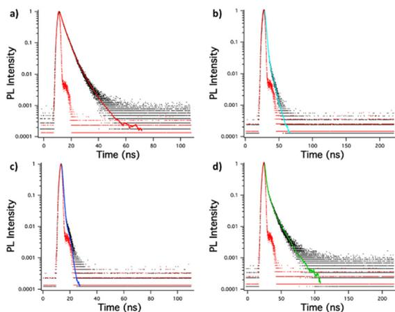
**Fig. 8** Singlet emission lifetime decay of (a) (MeOPh)<sub>2</sub>TTz, (b) (PrOPh)<sub>2</sub>TTz, (c) (BuOPh)<sub>2</sub>TTz, (d) (HepOPh)<sub>2</sub>TTz crystals.
