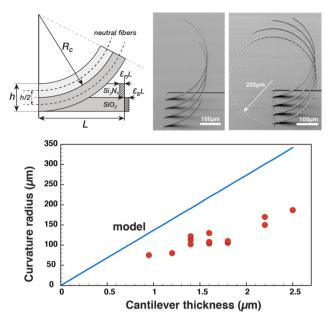
Fig. 3 (Top) Schematic of the analytical mechanical problem and SEM pictures of relaxed cantilever beams of increasing lengths (200 to 800  $\mu m$  by steps of 100  $\mu m$ , width 40  $\mu m$ ) showing the circular deformed shape as well as a measurement of the radius of curvature. (Bottom) Curvature radius vs. cantilever thickness, comparison between analytical model (blue line) and measurement (red dots).
