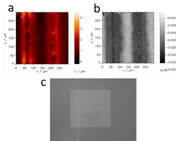
**Fig. 6** Hopping mode SECM images: topography (a), activity (b) and optical micrograph (c) of the ITO microband separated from the remaining ITO slide by laser-cutting. Scanning area:  $(300 \times 300) \mu\text{m}^2$ . The carbon microelectrode (SECM tip,  $\varnothing$  *ca.* 5.5  $\mu\text{m}$ ) is seen in the center of the optical image. Retracting distance: 10  $\mu\text{m}$ . Effective scanning rate: 3 image pixels per second. Electrolyte: aqueous 1 mM ferrocenemethanol in 0.1 M KCl.
