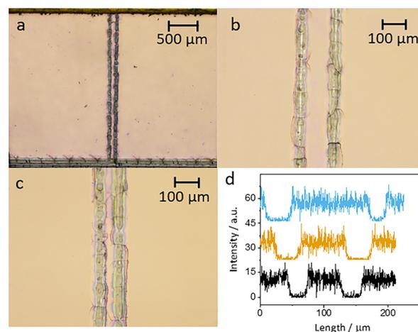
Fig. 4 Microscopy images of an electrode with a nominal width of 100  $\mu\text{m}$  at a) 2.5 $\times$  magnification and b) 10 $\times$  magnification, c) microscopy image of an electrode with a nominal width of 25  $\mu\text{m}$  at 10 $\times$  magnification, and d) EDX cross-section of the ITO electrodes depicting the intensity of indium.
