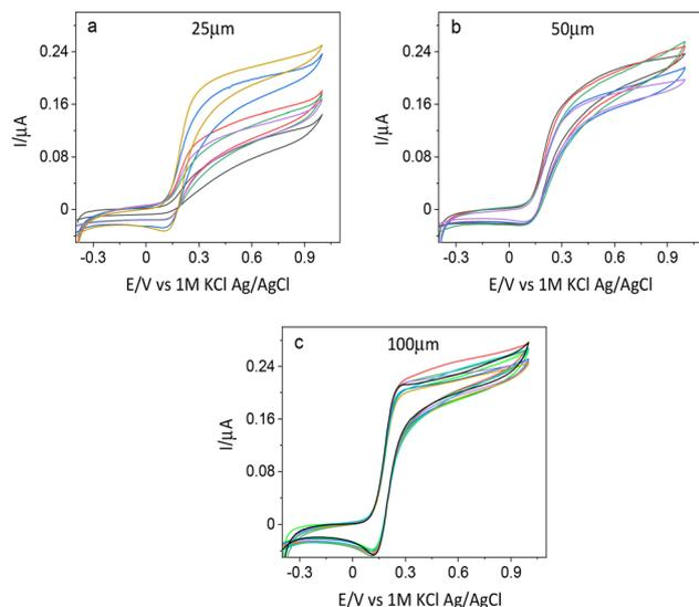
**Fig. 5** Cyclic voltammograms of electrodes of different sizes (a) 25, (b) 50 and (c) 100  $\mu\text{m}$  width, 2.5 mm length in 1 mM FcDM and 0.1 M  $\text{KNO}_3$  at 100  $\text{mV s}^{-1}$ . Each set of electrodes comes from the same plate.
