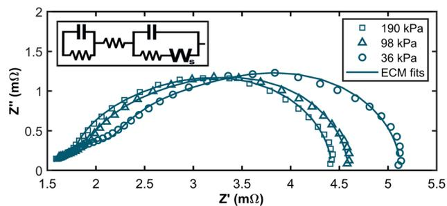
Fig. 4 Nyquist plot of the impedance spectra for hydrogen partial pressures of 36 kPa, 98 kPa, and 190 kPa. The experimental data points (markers) were recorded in a frequency range between 3 and 10 kHz at a current density of 1.0 A cm<sup>-2</sup>. The corresponding fits are displayed as solid curves. The ECM for fitting the impedance data is displayed in the top-left corner.
