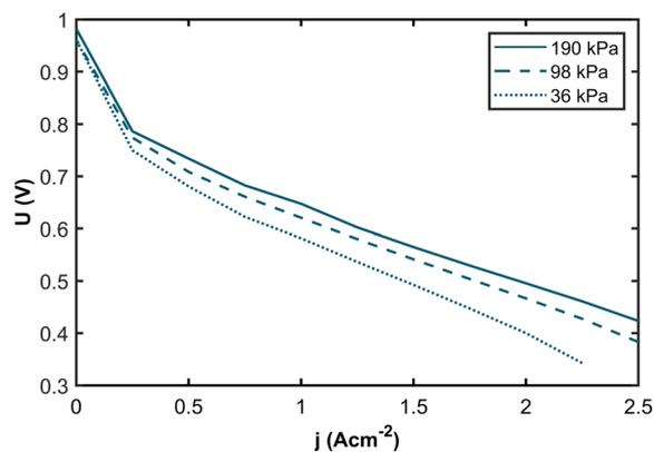
Fig. 2 Polarization curves for partial hydrogen pressures of 190 kPa (solid curve), 98 kPa (dashed curve), and 36 kPa (dotted curve). At 36 kPa, the maximum current density of  $2.5 \text{ A cm}^{-2}$  was not achieved without the cell voltage dropping below 0.3 V, which was specified as the lower voltage limit to ensure low degradation.
