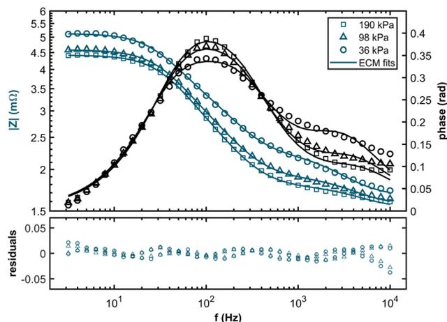
Fig. 5 Bode plot of the impedance spectra for hydrogen partial pressures of 36 kPa, 98 kPa, and 190 kPa. The experimental data points (markers) were recorded in a frequency range between 3 Hz and 10 kHz at a current density of  $1.0 \text{ A cm}^{-2}$ . The corresponding fits are displayed as solid curves. The corresponding relative residuals of the fits are displayed below.
