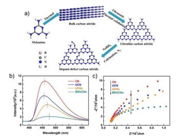
Fig. 6 (a) Schematic illustration of the synthesis protocol for the preparation of boron-doped defective ultrathin carbon nitride (BNUCN $_x$ ). (b) Steady state PL and (c) EIS spectra of different samples. Reproduced with permission from ref. 110. Copyright (2020) Elsevier.
