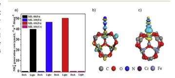
Fig. 7 (a) Photo-catalytic nitrogen fixation activity of different MIL MOFs. Charge density difference of a N<sub>2</sub> molecule adsorbed at (b) MIL-101(Cr) and (c) MIL-101(Fe). Reproduced with permission from ref. 131. Copyright (2020) Elsevier.
