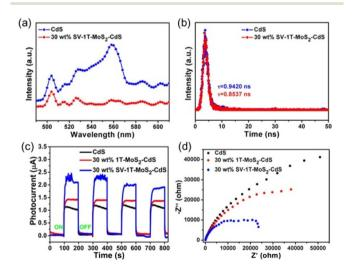
Fig. 5 (a) Steady state and (b) time-resolved PL spectra of CdS nanorods and 30 wt% SV-1T-MoS<sub>2</sub>/CdS composites at  $\lambda_{ex}$  = 405 nm. (c) Transient photo-current measurements and (d) EIS Nyquist plots of CdS nanorods, 30 wt% SV-1T-MoS<sub>2</sub>/CdS and 30 wt% 1T-MoS<sub>2</sub>/CdS composites. Reproduced with permission from ref. 93. Copyright (2020) American Chemical Society.
