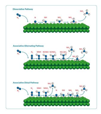
Fig. 1 Reaction pathways for the  $N_2$  reduction reaction to ammonia. Adapted with permission from ref. 18. Copyright (2017) Elsevier.
