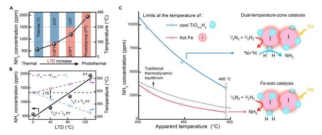
Fig. 9 (A) NH<sub>3</sub> concentration under combined solar irradiation and external heating by  $TiO_{2-x}H_y$ /Fe at a constant temperature of 495 °C. (B) NH<sub>3</sub> concentration as a function of the local temperature difference (LTD). (C) Comparison of equilibrium limits at the temperature of "cool"  $TiO_{2-x}H_y$  and "hot" Fe for photo-thermal ammonia synthesis on  $TiO_{2-x}H_y$ /Fe (1 atm). Reproduced with permission from ref. 155. Copyright (2019) Elsevier.
