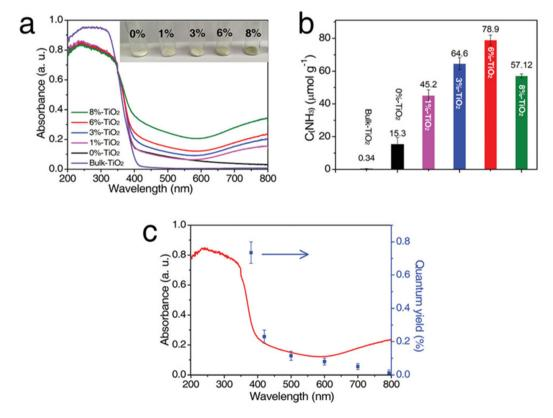
Fig. 4 (a) UV-vis diffuse reflectance spectra (DRS) of TiO<sub>2</sub> nanosheets with different percentages of Cu doping. (b) NH<sub>3</sub> yield of different TiO<sub>2</sub> nanosheets samples under UV-vis radiation (c) UV-vis diffuse reflectance spectrum and quantum efficiency for NH<sub>3</sub> evolution by 6%-TiO<sub>2</sub> sample under monochromatic light of different wavelengths. Reproduced with permission from ref. 65. Copyright (2019) John Wiley and Sons.
