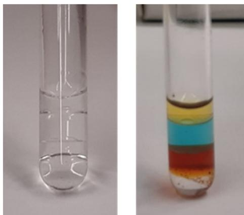
**Fig. 7** Left: the four-phase system of perfluorodecaline (bottom), LA-H,H, water, *n*-octane (top). Right: the same system after the addition of Cu(NO<sub>3</sub>)<sub>2</sub> and para red to make the phase separation more visible.
