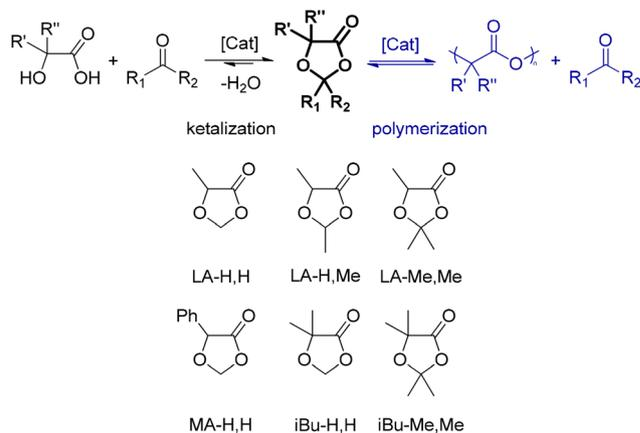
**Scheme 1** Formation of DOX through ketalization of  $\alpha$ -hydroxyacids (left); unwanted polycondensation (right); potential solvents studied in this work (bottom). Compound labelling: the first two letters refer to the parent acid (lactic: LA-; mandelic: MA-; and  $\alpha$ -hydroxyisobutyric: iBu-), and the following letters refer to the substituent groups at position 2 (-H and -Me). For example, in the case of 2,2,5-trimethyl-1,3-dioxolan-4-one, it is LA-Me,Me.
