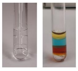
Fig. 7 Left: the four-phase system of perfluorodecaline (bottom), LA-H, H, water, n-octane (top). Right: the same system after the addition of Cu (NO<sub>3</sub>)<sub>2</sub> and para red to make the phase separation more visible.
