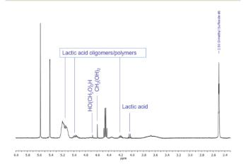
Fig. 6 Relevant portion of  $^1H$  NMR of LA-H,H treated with p-TsOH for 24 h at 100  $^{\circ}$ C.
