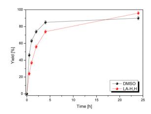
Fig. 5 Menschutkin kinetic profile in DMSO (black) and in LA-H,H (red).
