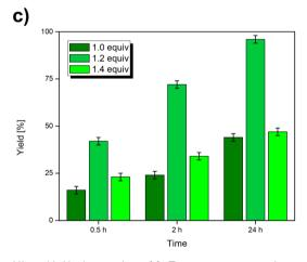
Fig. 4 Mizoroki–Heck reaction. (a) Temperature screening: phenyl iodide, 1 mmol; olefin, 1.2 mmol; and triethylamine, 1.2 mmol. (b) MR<sub>O</sub> screening: phenyl iodide, 1 mmol; triethylamine, 1.2 mmol; and olefin, 1 or 1.2 or 1.4 mmol. (c) MR<sub>B</sub> screening: phenyl iodide, 1 mmol; olefin, 1.2 mmol; and triethylamine, 1 or 1.2 or 1.4 mmol. Yield defined by  $^1\mathrm{H}$  NMR, error  $\pm 2\%$ .
