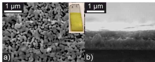
**Fig. 1** SEM micrographs of BiVO<sub>4</sub> photoelectrodes. (a) Plane view with photograph of a typical electrode, inset; and (b) cross section view.
