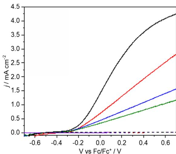
**Fig. 2** Linear sweep voltammograms of BiVO<sub>4</sub> photoelectrodes in electrolytes containing 2 M (black line), 1 M (red), 0.5 M (blue), 0.25 M (green), and 0.01 M (purple) PAA with 0.05 equiv. NEt<sub>3</sub>. Voltammograms were recorded in the dark (dashed) and under 450 nm LED illumination (solid). Scan rate 10 mV s<sup>-1</sup>.
