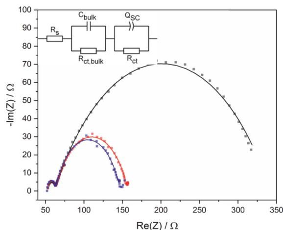
**Fig. 4** Nyquist plot and equivalent circuit for of an illuminated ( $450$  nm,  $32$   $\text{mW cm}^{-2}$ )  $\text{BiVO}_4$  photoanode in  $1$  M  $4\text{-Cl}$  PAA with  $0.05$  equiv.  $\text{Et}_3\text{N}$  at  $-0.26$  (grey circles),  $-0.06$  (red) and  $0.14$  V (blue). Data were acquired between  $500$  kHz– $50$  mHz, using an a.c. potential amplitude of  $10$  mV. Simulated impedance spectra are shown by the solid lines.
