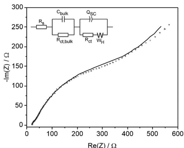
**Fig. 6** Nyquist plot and equivalent circuit for of an illuminated (450 nm, 32 mW cm<sup>-2</sup>) BiVO<sub>4</sub> photoanode in 0.05 M 4-Cl PAA solution with 0.05 equiv. Et<sub>3</sub>N containing 0.1 M TBAPF<sub>6</sub> supporting electrolyte at –0.06 V *vs.* Fc/Fc<sup>+</sup>. Data were acquired between 500 kHz–50 mHz, using an a.c. potential amplitude of 10 mV. Simulated impedance spectra are shown by the solid lines.
