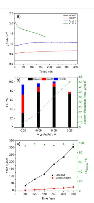
Fig. 3 (a) CPE of 1 M PAA with 0.05 equiv. Et<sub>3</sub>N at -0.26 (black), -0.08(red), +0.09 (blue) and +0.26 V (green) vs. Fc/Fc+; (b) faradaic efficiencies for bibenzyl (black), benzyl alcohol (red) and benzaldehyde (blue) as a function of electrolysis potential; (c) time-dependent bibenzyl (black) and benzyl alcohol (red) formation at +0.09 V vs. Fc/Fc<sup>+</sup> of 1 M PAA with 0.05 equiv. Et<sub>3</sub>N. Overall faradaic efficiency for bibenzyl is given in areen.
