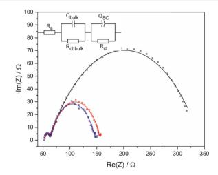
Fig. 4 Nyquist plot and equivalent circuit for of an illuminated (450 nm, 32 mW cm<sup>-2</sup>) BiVO<sub>4</sub> photoanode in 1 M 4-Cl PAA with 0.05 equiv. Et<sub>3</sub>N at -0.26 (grey circles), -0.06 (red) and 0.14 V (blue). Data were acquired between 500 kHz-50 mHz, using an a.c. potential amplitude of 10 mV. Simulated impedance spectra are shown by the solid lines.
