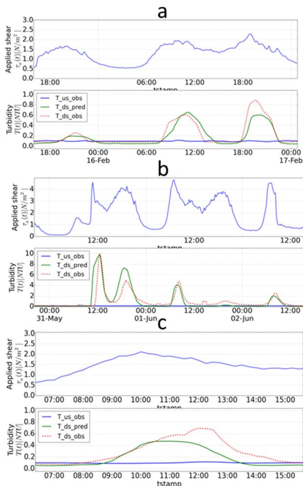
**Fig. 11** TM-2 event results from a 24 month simulation for TM-2. a) Burst in February 2016, b) burst in May–June 2016 c) burst in July 2016. Each sub figure top graph shows applied shear and bottom graph the modelled and measured turbidity response.
