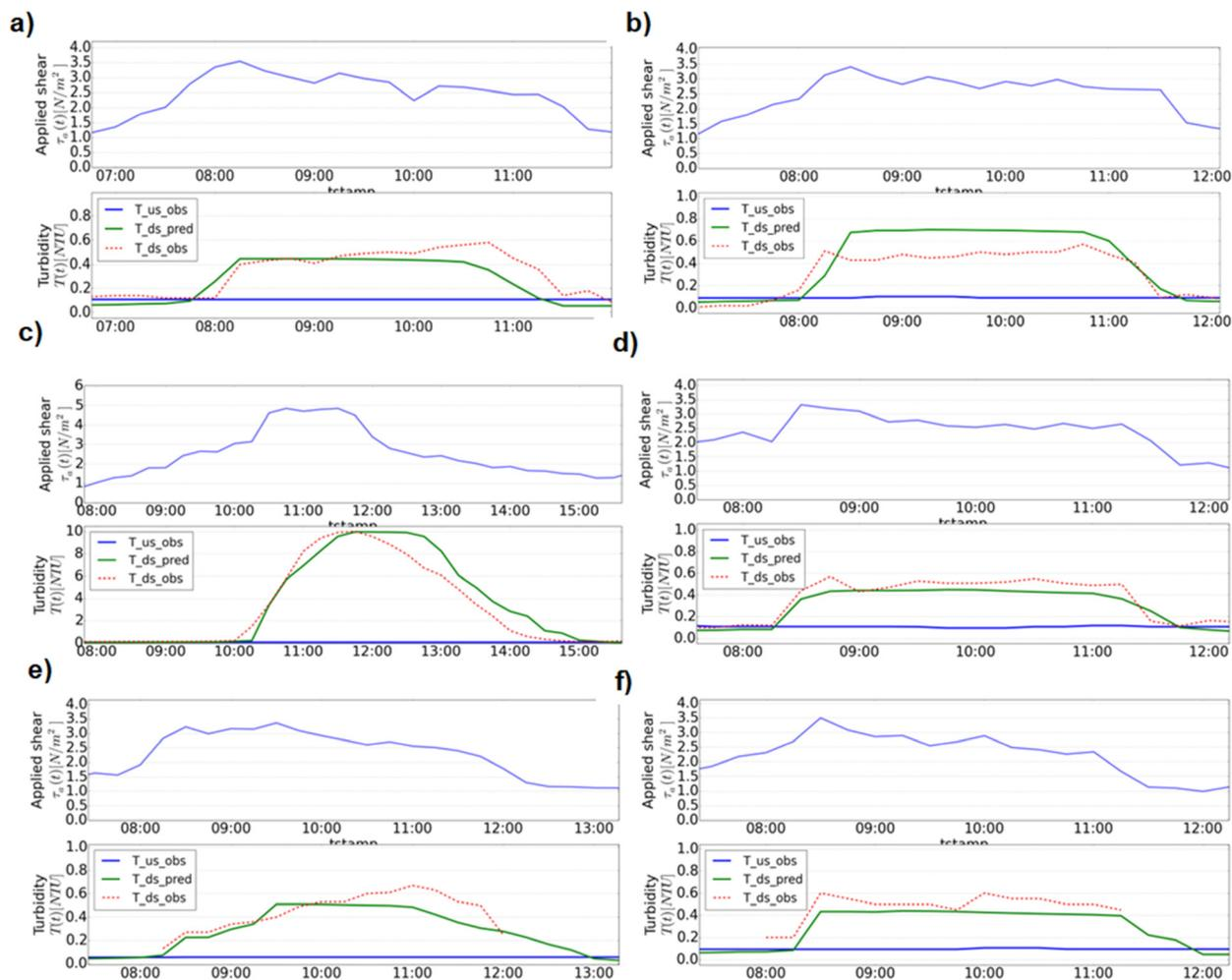
Fig. 9 TM-1 event results from a 24 month simulation for TM-1. a) Trial 1 b) trial 2 c) burst in March 2016 d) trial 3 e) trial 4 f) trial 5. Each sub figure top graph shows applied shear and bottom graph the modelled and measured turbidity response.
