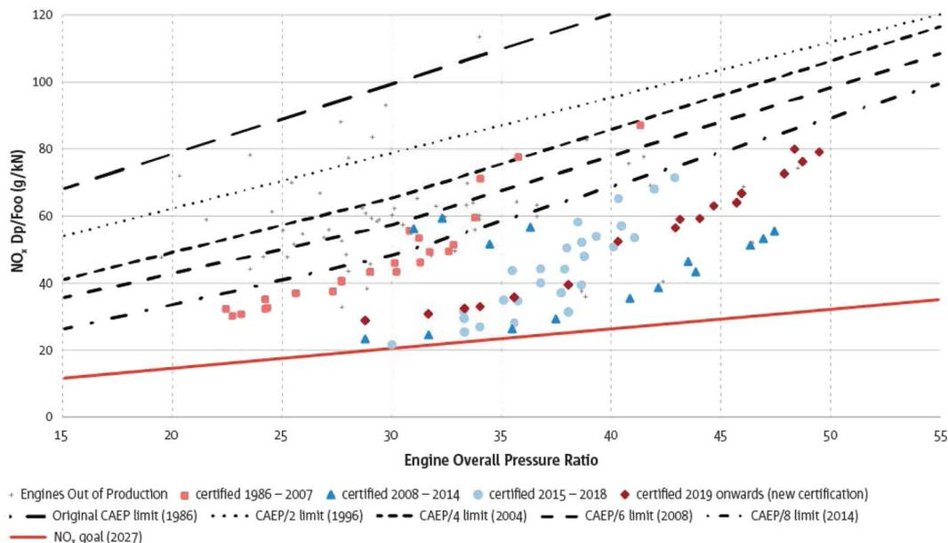
Fig. 2 Engine  $\text{NO}_x$  emissions certification data<sup>39</sup> showing the metric as ordinate and the pressure ratio as abscissa. The lines represent the various CAEP standards and goals.
