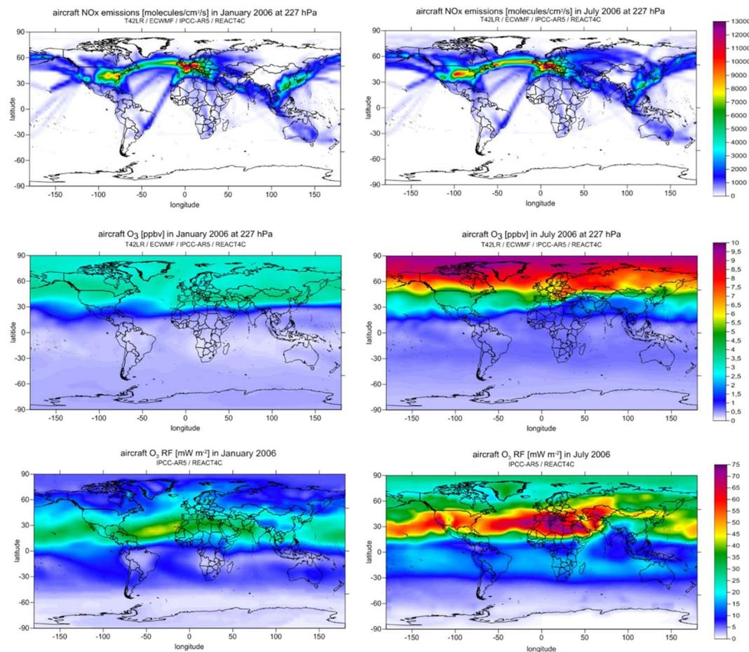
Fig. 9 Simulations of global aircraft  $\text{NO}_x$  emissions in 2006, January (upper left-hand panel), July (upper right-hand panel), ozone concentrations attributable to the aircraft  $\text{NO}_x$  at 227 hPa (approximately 11 km) (middle panels) in ppb, and the consequential radiative forcing (lower panels) (data replotted from simulations described by Skowron *et al.*, 2015).<sup>69</sup>
