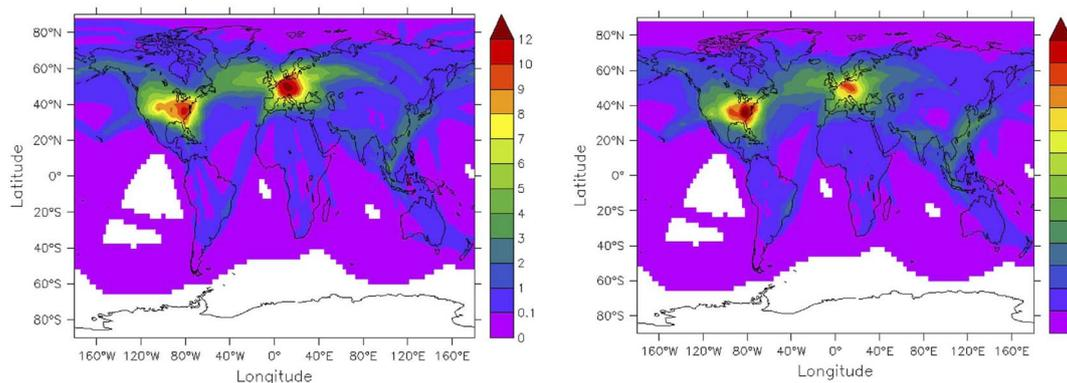
Fig. 8 Model simulation of the global distribution of contrail cirrus coverage associated with a visible optical thickness  $\geq 0.05$  in percent (left hand panel) and the net radiative forcing due to contrail cirrus in  $\text{mW m}^{-2}$  (right hand panel). Taken from Fig. 5 of Bier and Burkhardt (2022).<sup>61</sup>
