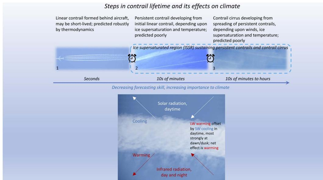
Fig. 7 The different timescales of contrail formation and potential transition to persistent contrails forming contrail cirrus. As shown in the lower panel, the net forcing is the residual of short wave and long wave radiation processes, which is time and space variant. In general contrails tend to have a net negative forcing during the day, and a net positive forcing at night, which is considered to dominate the overall time-integrated forcing (based on Shine and Lee, 2021).<sup>57</sup>
