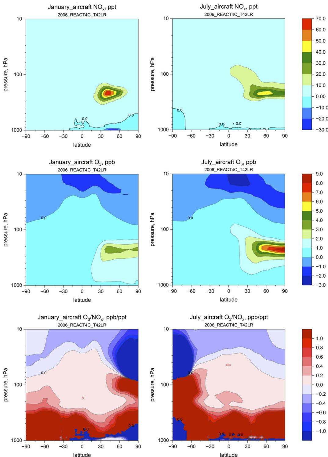
Fig. 10 Two-dimensional (latitude by height) averaged  $\text{NO}_x$  concentrations (VMR – volume mixing ratios) from aircraft (upper panels, left–right, Jan and July) in ppt, the resultant ozone concentration perturbations (middle panels) and the sensitivity of ozone to  $\text{NO}_x$  (ozone ppt/ $\text{NO}_x$  ppt). Data from Skowron *et al.* (2015)<sup>69</sup> simulations.
