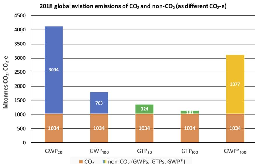
Fig. 20 Emissions from global aviation in 2018, expressed as Mtonnes of CO<sub>2</sub> and apparent emissions of non-CO<sub>2</sub>, expressed as various metrics and time horizons. The CO<sub>2</sub> emissions (orange) for 2018 are evidently invariant, whereas the non-CO<sub>2</sub>-e emission magnitude varies with metric (blue, GWP; green GTP, yellow GWP\*) and time horizon. Data from Lee *et al.* (2021).<sup>6</sup>
