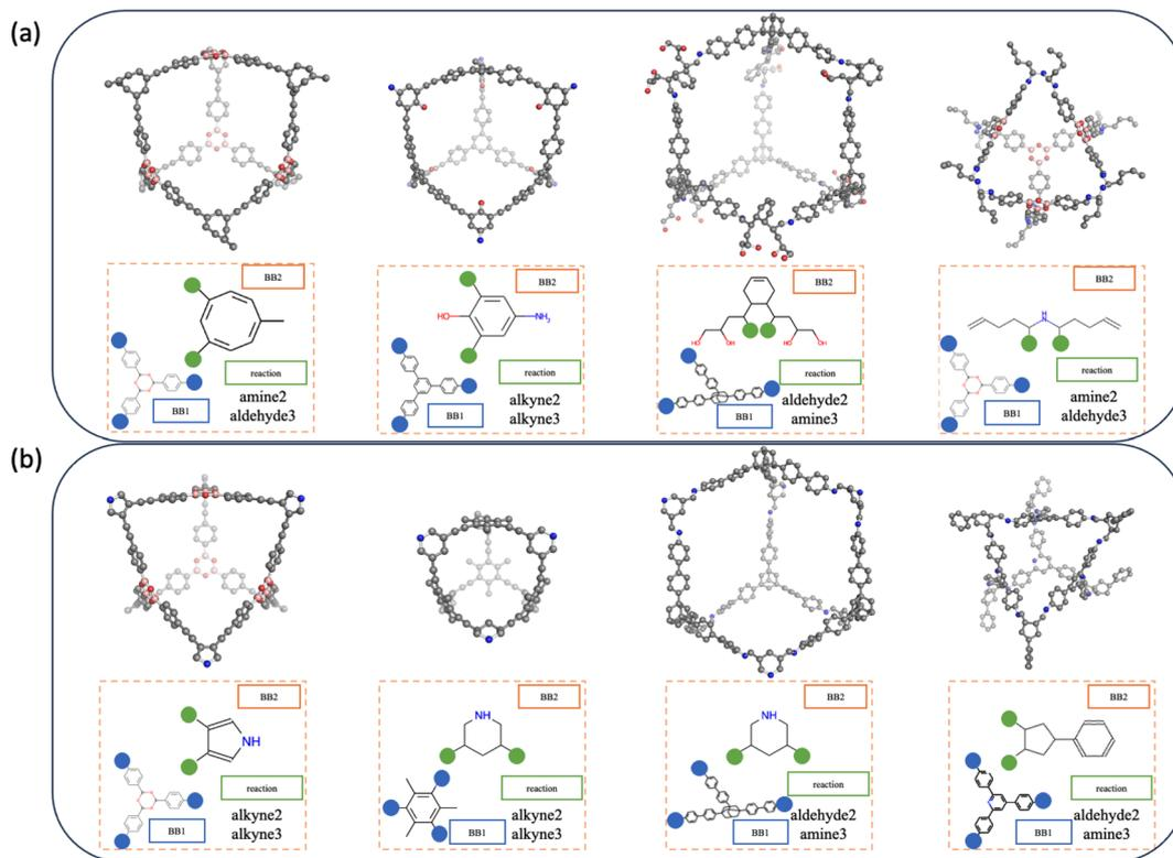
Fig. 7 Conformers and disassembled representations of a selection of generated shape-persistent POCs via (a) Bayesian optimisation starting from a training set molecule and (b) *slerp* between randomly selected molecules in the training set that have a threshold of probability of prediction above 80%. All molecular conformations and shape persistence were validated by MD simulations.
