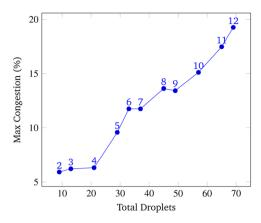
Fig. 19 Total droplets vs. Max Congestion. This data was obtained by running the simulation at a constant grid size of  $45 \times 45$  over a range of gene lengths two to twelve. The number above each point represents the gene length. The vertical axis displays the total congestion and the horizontal axis displays the total amount of droplets pulled from reservoirs to synthesize the gene. The relationship between the number of pulled droplets and the maximum congestion is approximately linear.
