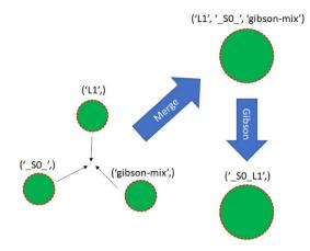
Fig. 13 Three single-species droplets merge, becoming a larger droplet with mixed species. The droplet undergoes Gibson assembly, becoming a different species
