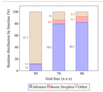
Fig. 16 Runtime distribution by major function. This data was obtained by running the simulation at an approximately constant congestion ratio. Here the congestion ratio is the total number of droplets pulled from reservoirs divided by the number of grid points. The approximate constant congestion ratio used was 0.0036 droplets gridsize<sup>-2</sup> which was chosen by convenience. The parameters for these trials are shown in 2.
