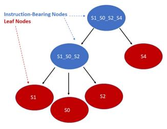
Fig. 11 Simplified diagram of a small assembly tree data structure. In red, the leaf nodes each contain a single symbol. The root node represents the final desired symbol sequence or gene. Non-leaf nodes contain assembly instructions readable by the manager. We note that the linkers between the symbols have been excluded for readability. See Fig. 12 for more details on individual nodes.
