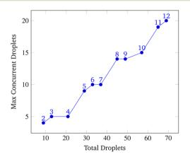
Fig. 17 Max Concurrent droplets vs. total droplets. This data was obtained by running the simulation at a constant grid size of  $45\times45$  over a range of gene lengths two to twelve. The number above each point represents the gene length. The vertical axis displays the maximum number of droplets recorded on the chip during the entirety of the simulation while the horizontal axis displays the total amount of droplets pulled from reservoirs to synthesize the gene.
