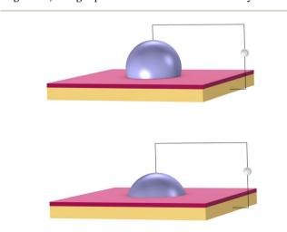
Fig. 3 Electrowetting: aqueous droplets spread when a voltage is applied between a droplet and an insulating electrode (shown in orange). The droplet rests upon a hydrophobic dielectric (shown in red). Top: no voltage. Bottom: high voltage.
