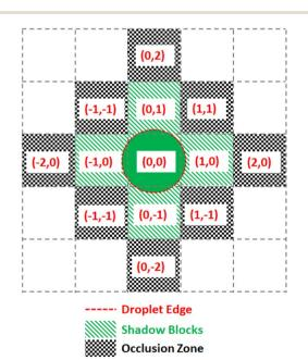
Fig. 9 Diagram of the digitization of droplet shadow and occlusion zones. A droplet centered on a grid space with relative coordinates (0, 0) has a sufficient radius to touch the four nearest neighboring grid spaces, making five shadow blocks. All grid spaces adjacent to the shadow blocks are designated as occlusion zones.
