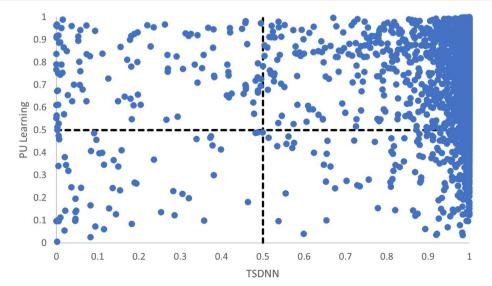
Fig. 4 Scatter plot of our TSDNN predicted scores vs. PU learning on ICSD materials from the test set. This shows that the PU learning method falsely classified many more materials as negative (Quadrant IV) than our TSDNN model (Quadrant II) for the PU learning predictions.
