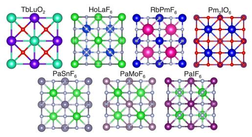
Fig. 6 The discovered new crystal structures with zero  $E_{\text{bull}}$ .
