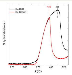
Fig. 2 NH<sub>3</sub> temperature-programmed desorption profiles of Ru/CaO and Ru-K/CaO catalysts after reduction at 500 °C.
