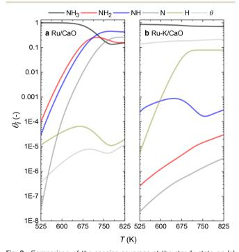
Fig. 9 Comparison of the species coverage at the steady state on (a) Ru/CaO; Case C (NH dissociation) and (b) Ru-K/CaO; Case A (NH<sub>3</sub> dissociation) as the rate-determining steps, respectively.
