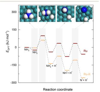
Fig. 3 Potential energy surface profile of the dehydrogenation of NH<sub>v</sub> (y = 1-3) on Ru(111) and the corresponding transition states and Ru-K/ CaO(111). The respective transition states of which are depicted in Fig. 4.
