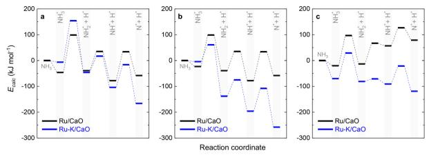
Fig. 10 Potential surface diagrams considering the obtained activation energies from the fitted models: (a) Case A (NH<sub>3</sub> dissociation); (b) Case B (N<sub>2</sub> desorption); and (c) Case C (NH dissociation).
