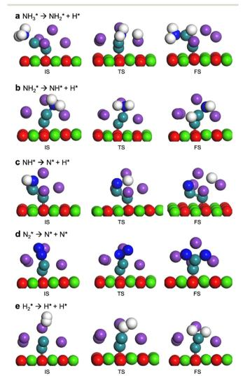
Fig. 4 Optimized structures of the initial, transition, and final states on the Ru-K/CaO(111) surface.
