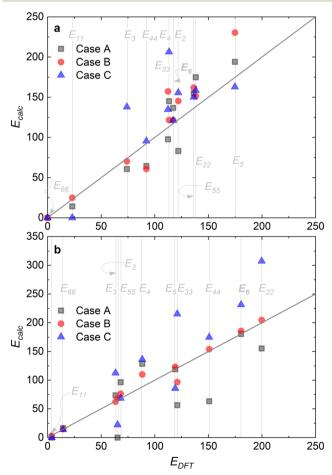
Fig. 8 Comparison via parity plots of the DFT-calculated activation energies ( $E_{DFT}$ ) and those predicted via fitting ( $E_{calc}$ ): (a) Ru/CaO; (b) Ru-K/CaO
