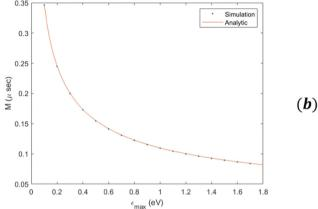
Fig. 4 (a) The final position on the detector as a function of the initial velocity, for electrons that are starting from the origin with initial velocity on y axis only, for different values of  $\varepsilon_{\text{max}}$ . The continuous lines are given by the analytical derivation and the dots are given by the simulation. (b) The magnification as a function of  $\varepsilon_{max}$ .
