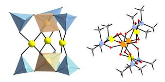
Fig. 1 Combined ball-and-stick/polyhedral representation and Ball-and-stick representation (side view) of 1. Color code:  $\{PtO_6\}$  orange octahedra,  $\{(CH_3)_2AsO_2\}$  blue tetrahedra, Au yellow atoms. Pt orange, Au yellow, As sky blue, O red, C grey. Hydrogen atoms omitted for clarity.
