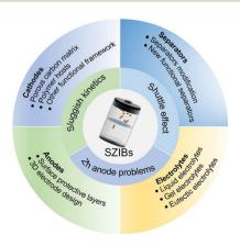
Fig. 1 Overview of challenges in and improved strategies for constructing aqueous zinc-iodine batteries.
