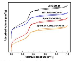
Fig. 5 N<sub>2</sub> adsorption isotherms of fresh and spent catalysts.
