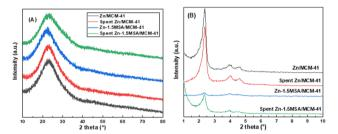
Fig. 6 Wide angle XRD patterns (A) and small angle XRD patterns (B) of the fresh and used catalysts.
