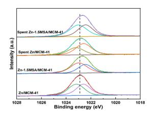
Fig. 8 Zn 2p<sub>3/2</sub> XPS pattern of the fresh and used catalysts.
