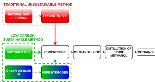
Fig. 8 Block diagram illustrating the traditional and renewable (pure H<sub>2</sub> with captured CO<sub>2</sub>) methods of methanol production. Modified after ref. 76.
