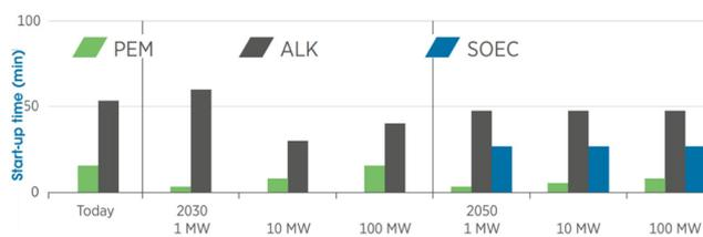
Fig. 5 Comparison of start-up times for PEM, alkaline (ALK), and solid oxide electrolyzer cell (SOEC) technologies.<sup>50</sup>
