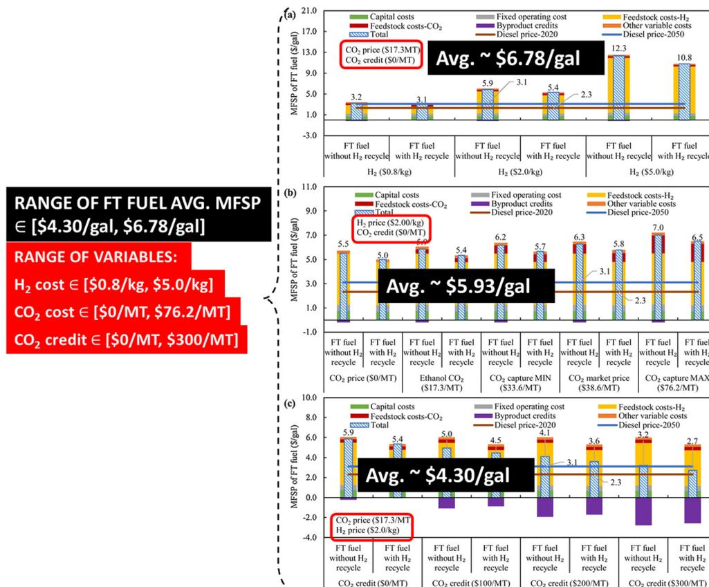
Fig. 17 MFSP of SAF (FT fuel) as a function of the H<sub>2</sub> production cost, CO<sub>2</sub> cost, and the credit for saved carbon for a production capacity of 351 MT per day (divided among 90 MT per day of naphtha, 164 MT per day of jet fuel, and 97 MT per day of diesel). Adapted from ref. 99.
