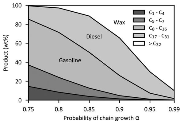
Fig. 15 Probabilistic distribution of the hydrocarbon products with different carbon chain lengths in the Fischer–Tropsch (FT) process.<sup>97</sup>
