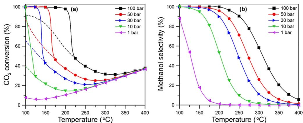
Fig. 10 Sensitivity of methanol synthesis (from  $\text{CO}_2$  and  $\text{H}_2$ ) as a function of pressure and temperature.<sup>77,86</sup>
