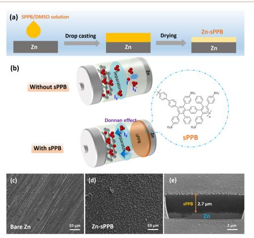
Fig. 1 (a) Scheme of the sPPB coating process on Zn metal; (b) mechanism of Zn-I<sub>2</sub> batteries with bare Zn and sPPB protected Zn as anodes. SEM images of (c) the bare Zn, (d) top-view of sPPB protected Zn, and (e) cross-section-view of sPPB coated Zn.
