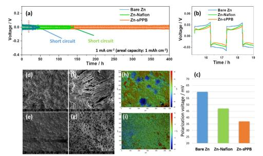
Fig. 2 (a) The cycling performance of bare Zn, Zn-Nafion, Zn-sPPB at 1 mA cm<sup>-2</sup> with areal capacity of 1 mA h cm<sup>-2</sup>; (b and c) the comparison of Zn plating/stripping profiles and the polarization voltage values for bare Zn, Zn-Nafion, and Zn-sPPB electrodes between 15-19 h. (d-i) SEM, and height mapping images of (d, f and h) bare Zn after 40 h cycling and (e, g and i) Zn-sPPB after 80 h cycling in the symmetrical cells
