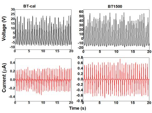
Fig. 7 Mechanical energy harvesting performance of the BT-cal/PDMS and BT1500/PDMS composite-based PEH devices under the periodic mechanical load of 5 N. Top panel shows the scavenged open circuit voltage (V<sub>oc</sub>) and bottom panel shows the scavenged short circuit current (I<sub>sc</sub>) for the devices
