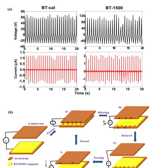
Fig. 8 (a) Mechanical energy harvesting performance of BT-cal/PDMS and BT1500/PDMS composite based hybrid (PEH + TEH) devices under the periodic mechanical load of 5 N. Top panel shows the scavenged open circuit voltage ( $V_{\infty}$ ) and bottom panel shows the scavenged short circuit current  $(I_{sc})$  for the devices. Inset shows the real hybrid device. (b) Schematic working mechanism of the TEH device.
