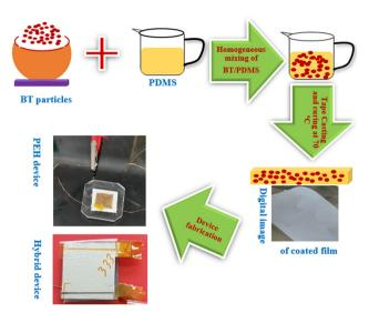
Fig. 5 Processing steps of the BaTiO<sub>3</sub> piezoceramic/PDMS composite and PEH/hybrid (PEH + TEH) device fabrication.
