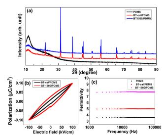
Fig. 6 (a) XRPD on the surface of the BaTiO<sub>3</sub> piezoceramics/PDMS composite showing the signature of the polymer (broad hump) and ceramic particle present in the film. (b) P-E hysteresis loops for the composites. (c) Dielectric permittivity ( $\varepsilon'$ ) of the composite specimens as a function of frequency
