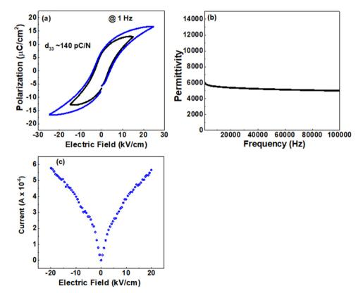
Fig. 3 (a) Bipolar polarization (P) – electric field (E) hysteresis curve for the BT-1500 pellet. (b) Dielectric permittivity (ε') of the BT-1500 pellet specimen. (c) Leakage current (I) vs. electric field (E) of BT-1500
