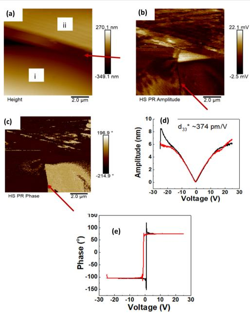
Fig. 4 Piezoresponse Force Microscopy (PFM) studies on the BT-1500 pellet – (a) Surface topography, where the arrow indicates the grain boundary region; parts of two grains are indicated with numbers. (b) and (c) PFM amplitude and phase images at zero bias voltage, where arrows indicate the domain wall boundary; (d) and (e) PFM amplitude and phase under different bias voltage. Converse piezoelectric coefficient ( $d_{33}^*$ ) determined from the slope at the linear region in (d).
