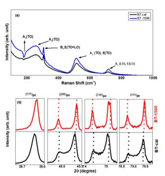
Fig. 2 (a) Comparative Raman spectra for different BaTiO<sub>3</sub> specimens (BT-1500 and BT-cal respectively). Each vibrational mode is indicated by the arrows. (b) X-Ray powder diffraction (XRPD) Bragg profiles of different BaTiO<sub>3</sub> specimens. Dotted lines indicate polar structural distortion for the specimens. Each pair of Bragg peaks is plotted for the same  $2\theta$  interval.
