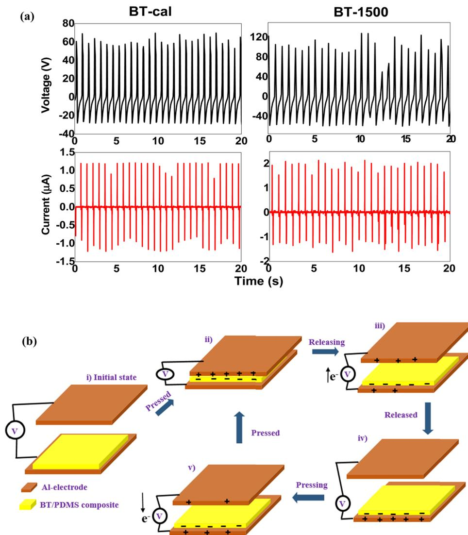
**Fig. 8** (a) Mechanical energy harvesting performance of BT-cal/PDMS and BT1500/PDMS composite based hybrid (PEH + TEH) devices under the periodic mechanical load of 5 N. Top panel shows the scavenged open circuit voltage ( $V_{oc}$ ) and bottom panel shows the scavenged short circuit current ( $I_{sc}$ ) for the devices. Inset shows the real hybrid device. (b) Schematic working mechanism of the TEH device.
