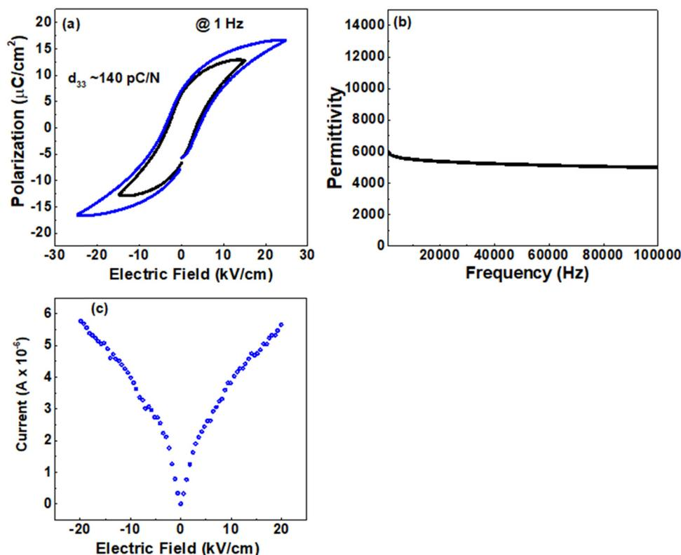
Fig. 3 (a) Bipolar polarization ( $P$ ) – electric field ( $E$ ) hysteresis curve for the BT-1500 pellet. (b) Dielectric permittivity ( $\epsilon'$ ) of the BT-1500 pellet specimen. (c) Leakage current ( $I$ ) vs. electric field ( $E$ ) of BT-1500.
