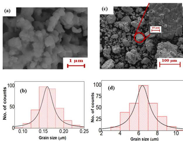
Fig. 1 (a) Scanning electron microscopy (SEM) micrograph of a calcined powder of BaTiO<sub>3</sub> (BT-cal). (b) The corresponding grain size distribution is shown in the histogram. (c) SEM micrograph of the crushed and annealed powder of the sintered specimen of BaTiO<sub>3</sub> (BT-1500) showing clustering of the grains with varying size. The inset shows the actual grainy contrast of the sintered pellet. (d) The grain size distribution of the sintered pellet is shown in the histogram.
