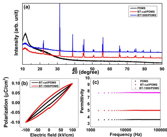
Fig. 6 (a) XRPD on the surface of the  $\text{BaTiO}_3$  piezoceramics/PDMS composite showing the signature of the polymer (broad hump) and ceramic particle present in the film. (b)  $P$ - $E$  hysteresis loops for the composites. (c) Dielectric permittivity ( $\epsilon'$ ) of the composite specimens as a function of frequency.
