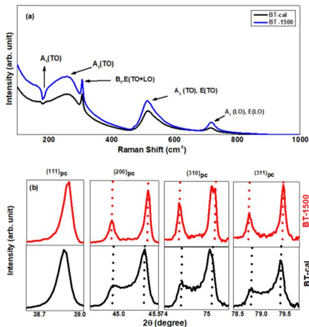
Fig. 2 (a) Comparative Raman spectra for different  $\text{BaTiO}_3$  specimens (BT-1500 and BT-cal respectively). Each vibrational mode is indicated by the arrows. (b) X-Ray powder diffraction (XRPD) Bragg profiles of different  $\text{BaTiO}_3$  specimens. Dotted lines indicate polar structural distortion for the specimens. Each pair of Bragg peaks is plotted for the same  $2\theta$  interval.
