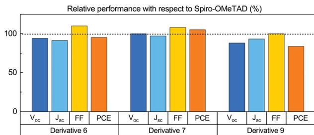
Fig. 3 Average  $V_{oc}$ ,  $J_{sc}$ , FF and PCE of PSCs prepared with derivatives **6**, **7** and **9**, with respect to the average values obtained for reference devices prepared using Spiro-OMeTAD as the HTL.
