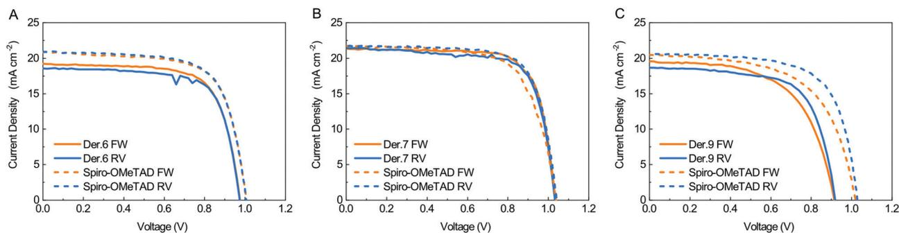
Fig. 2  $J$ - $V$  graphs for the best PSCs obtained using derivatives 6 (graph A), 7 (graph B) and 9 (graph C) as the HTL. In each graph, both the forward (orange) and reverse (blue) scan are shown, for both the chosen derivative (full line) and a reference PSC (dashed line) produced using Spiro-OMeTAD as the HTL.
