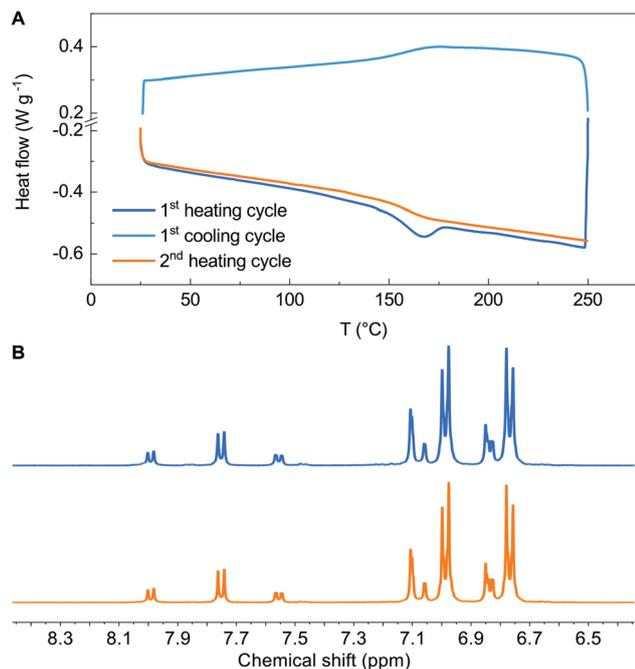
Fig. 1 (A) DSC characterization of derivative 7. (B) Details of the aromatic portion of the  $^1\text{H}$  NMR spectra in  $\text{THF-}d_8$  of derivative 7 before (blue line) and after (orange line) the DSC thermal treatment.
