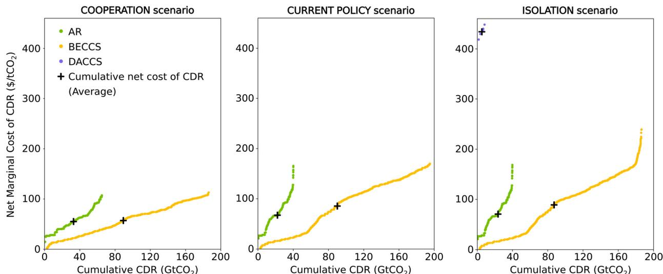
**Fig. 18** Cost supply curves of each CDR option deployed by 2100, under alternative P3-consistent policy scenarios. BECCS delivers the most cost-efficient CDR – its cost supply curve is below all the ones of the other CDR options – and therefore the most CDR, and that in all scenarios.
