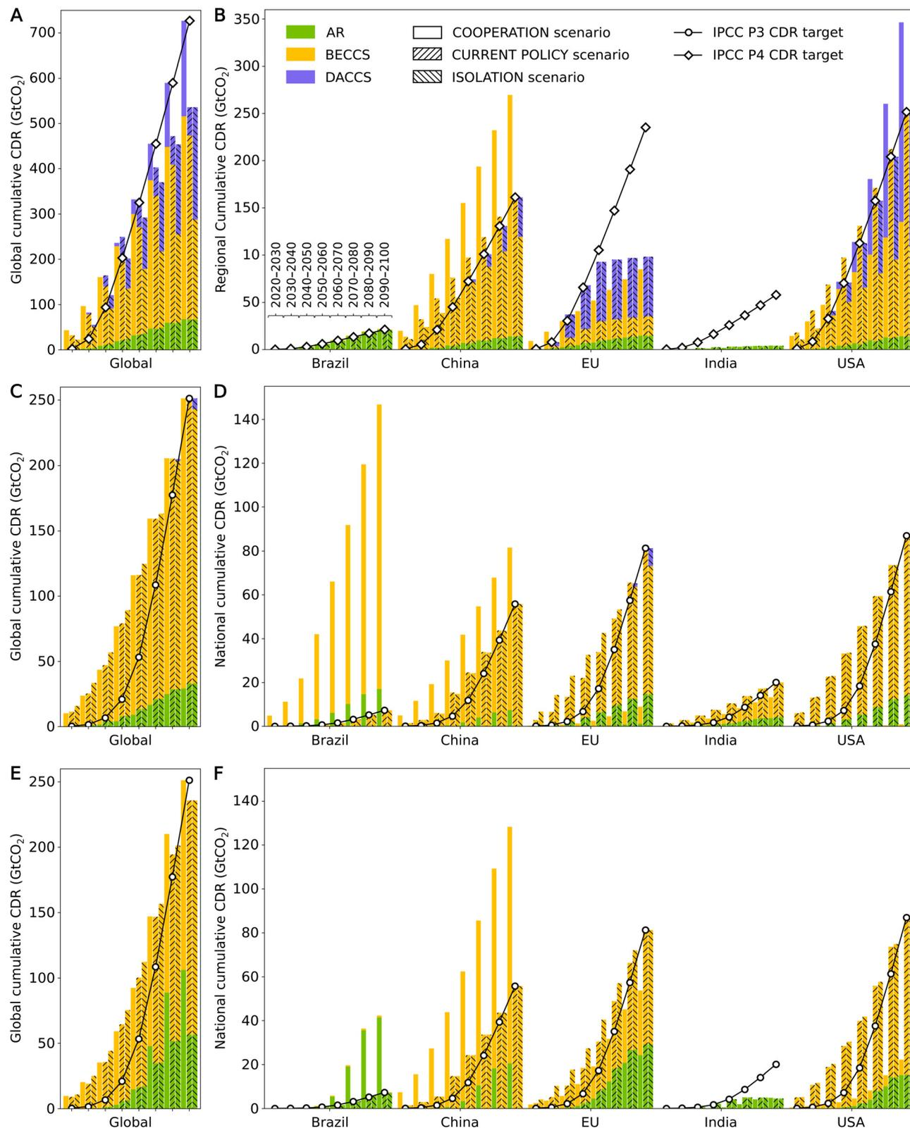
Fig. 19 Sensitivity analysis are performed on: increasing CDR targets, globally (A) and nationally (B); increasing CO<sub>2</sub> storage availability, globally (C) and nationally (D); and on increasing built (*i.e.*, BECCS and DACCS) and expansion (*i.e.*, AR) rates, globally (E) and nationally (F).
