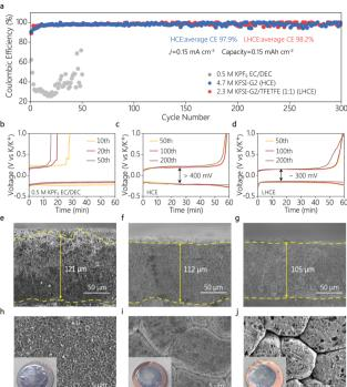
Fig. 3 (a) Cycling performances of K|Cu coin cells and the corresponding voltage profiles in (b) 0.5 M KPF<sub>6</sub> EC/DEC electrolyte, (c) HCE and (d) LHCE at 0.15 mA cm $^{-1}$ . (e-g) Cross-sectional and (h-j) top-view SEM images of K deposition morphologies in (e and h) 0.5 M KPF<sub>6</sub> EC/DEC, (f and i) HCE and (g and j) LHCE. Optical images of K deposits on Cu foil are shown in the inset of h-i. The capacity of K metal on the Cu substrate was  $4.0 \text{ mA h cm}^{-2}$ .
