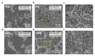
Fig. 4 Top-view SEM images of K deposition morphologies in (a-c) HCE and (d-f) LHCE with enlarged views (c and f) at a current density of (a and d)  $0.05 \text{ mA cm}^{-2}$  and (b and e)  $0.5 \text{ mA cm}^{-2}$  with a capacity of 0.15 mA h cm<sup>-2</sup>
