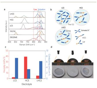
Fig. 2 (a) Raman spectra of LCE, HCE and LHCE. (b) Schematic illustration of the solvation structure of LCE, HCE and the diluted LHCE. (c) Viscosity and ionic conductivity of LCE, HCE and LHCE. (d) Contact angles and wettability tests between the separator and different electrolytes.
