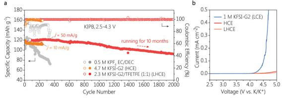
Fig. 1 (a) Cycling performance of K|PB batteries in 0.5 M KPF<sub>6</sub> EC DEC electrolyte at 50 mA  $g^{-1}$ , HCE at 10 mA  $g^{-1}$ , and LHCE at 50 mA  $g^{-1}$ . (b) LSV of various concentrations of KFSI/G2 electrolytes in K|Al coin cells with Al as the working electrode and K metal as the counter electrode. The scan rate is  $0.5 \text{ mV s}^{-1}$
