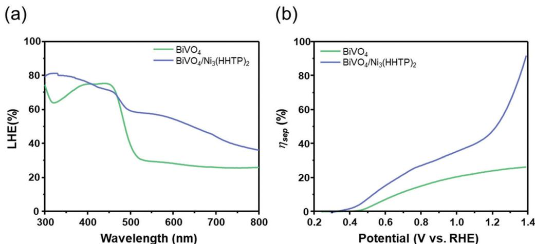
Fig. 5 (a) Light harvesting efficiency (LHE) (%) and (b) charge separation efficiency ( $\eta_{sep}$ ) of BiVO<sub>4</sub> and BiVO<sub>4</sub>/Ni<sub>3</sub>(HHTP)<sub>2</sub>.
