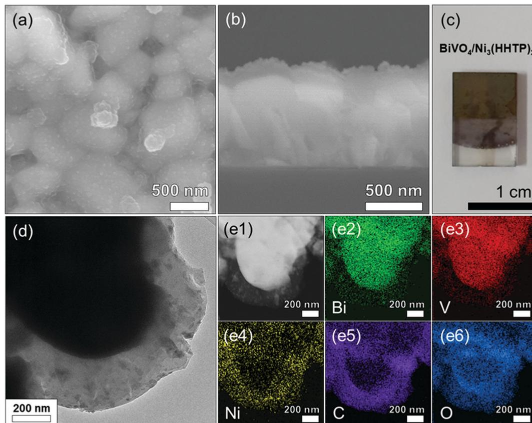
Fig. 2 (a) Top-view and (b) cross-sectional view of the SEM image of  $\text{BiVO}_4/\text{Ni}_3(\text{HHTP})_2$  heterostructure (solvothermal reaction for 3.5 h). (c) Photograph of  $\text{BiVO}_4/\text{Ni}_3(\text{HHTP})_2$  heterostructure photoanode. (d) TEM image and (e1–6) elemental mappings of  $\text{BiVO}_4/\text{Ni}_3(\text{HHTP})_2$  heterostructure.
