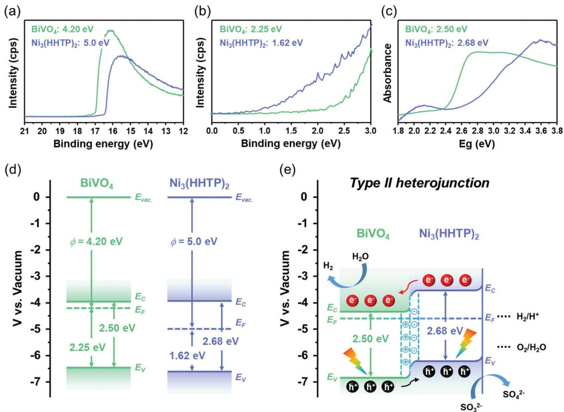
Fig. 4 UPS of BiVO<sub>4</sub> and BiVO<sub>4</sub>/Ni<sub>3</sub>(HHTP)<sub>2</sub> for obtaining (a) work function ( $\phi$ ) and (b) VBM. (c) UV-vis spectra of BiVO<sub>4</sub> and BiVO<sub>4</sub>/Ni<sub>3</sub>(HHTP)<sub>2</sub>. Schematic energy band diagram of BiVO<sub>4</sub> and BiVO<sub>4</sub>/Ni<sub>3</sub>(HHTP)<sub>2</sub> (d) before contact and (e) after contact.
