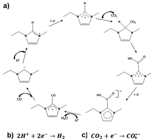
**Fig. 6** Mechanism for electrochemical activation of CO<sub>2</sub> by 1-ethyl-3-methyl imidazolium based on the mechanism proposed by Wang *et al.*<sup>28</sup>
