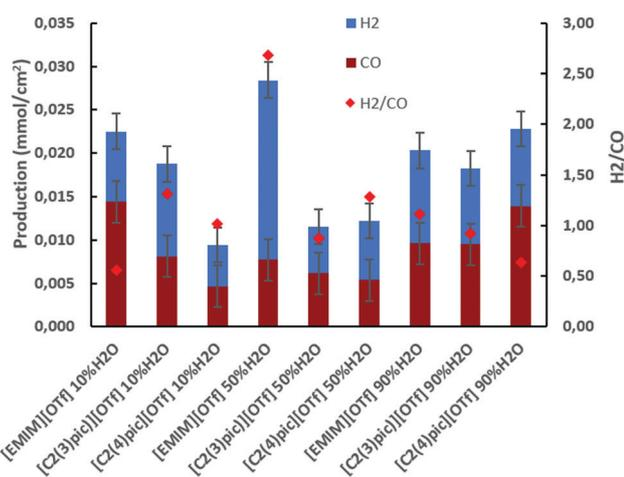
Fig. 4 Electrolysis on Zinc cathodes at 45 °C, 10 bar CO<sub>2</sub> applied current density in the range of  $-0.65$  to  $-0.85$  mA cm<sup>-2</sup> and 10 C of charge passed.
