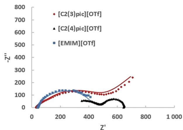
**Fig. 10** EIS on the Zn cathodes in a solution of 50 wt% water an ionic liquid at 10 bar CO<sub>2</sub> with an applied potential of  $-1.4$  V vs. Ag/Ag<sup>+</sup> (QRE); the continuous line corresponds to the fitting.
