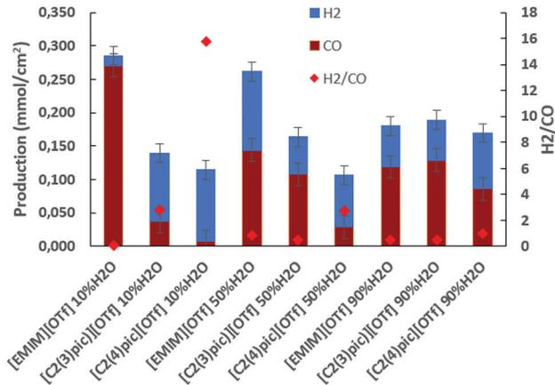
Fig. 5 Electrolysis on Zinc cathodes at 45 °C, 10 bar CO<sub>2</sub> applied current density of  $-7$  mA cm<sup>-2</sup> and 50 C of charge passed.
