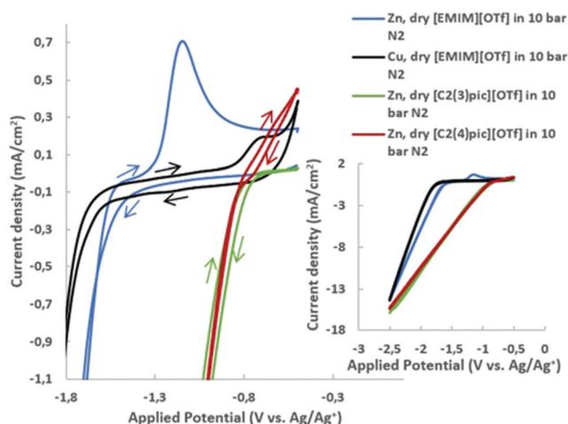
Fig. 2 Cyclic voltammograms at 45 °C carried out at 50 mV s<sup>-1</sup> in the potential range of -0.5 V up to -2.5 V vs. Ag/Ag<sup>+</sup> (QRE) in dry [EMIM][OTf] at zinc and copper cathodes and in dry [C<sub>2</sub>(3)pic][OTf] and [C<sub>2</sub>(4)pic][OTf] at zinc cathodes in N<sub>2</sub> atmosphere.
