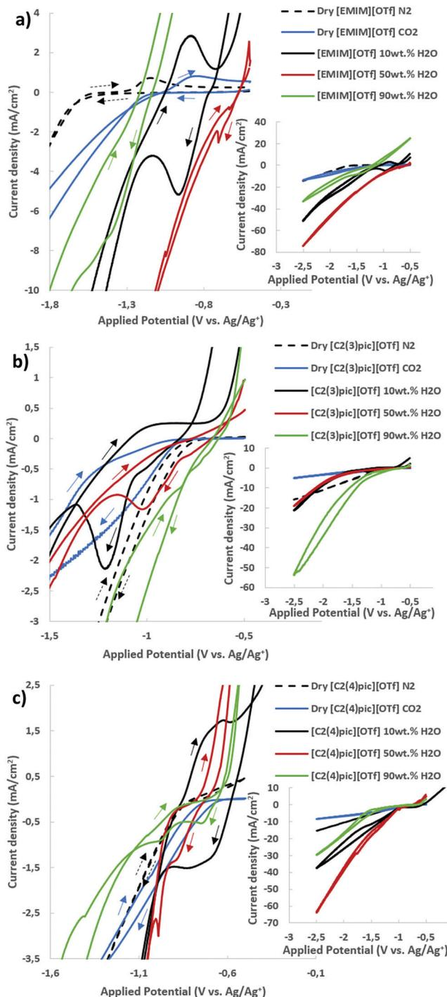
Fig. 3 Cyclic voltammograms on zinc cathodes at  $45 \text{ }^\circ\text{C}$  carried out at  $50 \text{ mV s}^{-1}$  in the potential range of  $-0.5 \text{ V to } 2.5 \text{ V vs. Ag/Ag}^+$  (QRE) for the ionic liquids  $[\text{EMIM}][\text{OTf}]$ ,  $[\text{C}_2(3)\text{pic}][\text{OTf}]$  and  $[\text{C}_2(4)\text{pic}][\text{OTf}]$  with different compositions of water in  $\text{CO}_2$  atmosphere and dried in  $\text{N}_2$  atmosphere at 10 bar.
