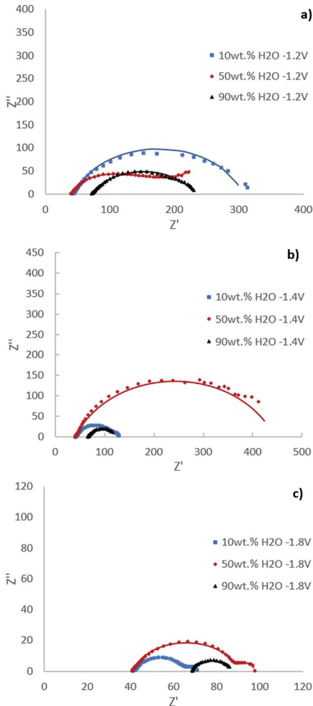
Fig. 8 EIS on the Zn cathodes of the EMIMOTf electrolytes with different water compositions at 10 bar  $\text{CO}_2$  with different applied potential: (a)  $-1.2$  V vs.  $\text{Ag}/\text{Ag}^+$  (QRE), (b)  $-1.4$  V vs.  $\text{Ag}/\text{Ag}^+$  (QRE), (c)  $-1.8$  V vs.  $\text{Ag}/\text{Ag}^+$  (QRE); the continuous line corresponds to the fitting.
