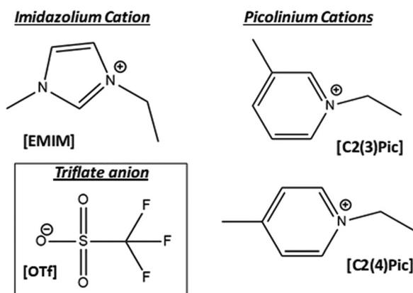
Fig. 1 Chemical structures of the ILs used in this work: 1-ethyl-3-methyl-imidazolium cation [EMIM]<sup>+</sup>; 1-ethyl-4-picolinium cation [C<sub>2</sub>(4)pic]<sup>+</sup>; 1-ethyl-3-picolinium cation [C<sub>2</sub>(3)pic]<sup>+</sup> combined with trifluoromethanesulfonate anion [OTf]<sup>−</sup>.
