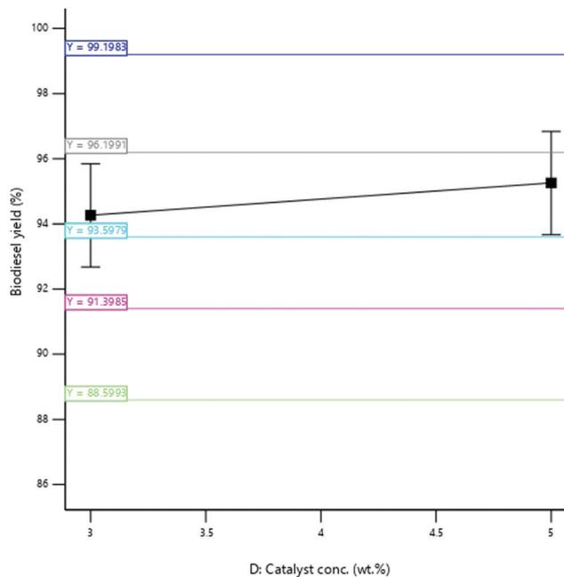
Fig. 13 Effect of the catalyst concentration on the shea butter biodiesel yield.
