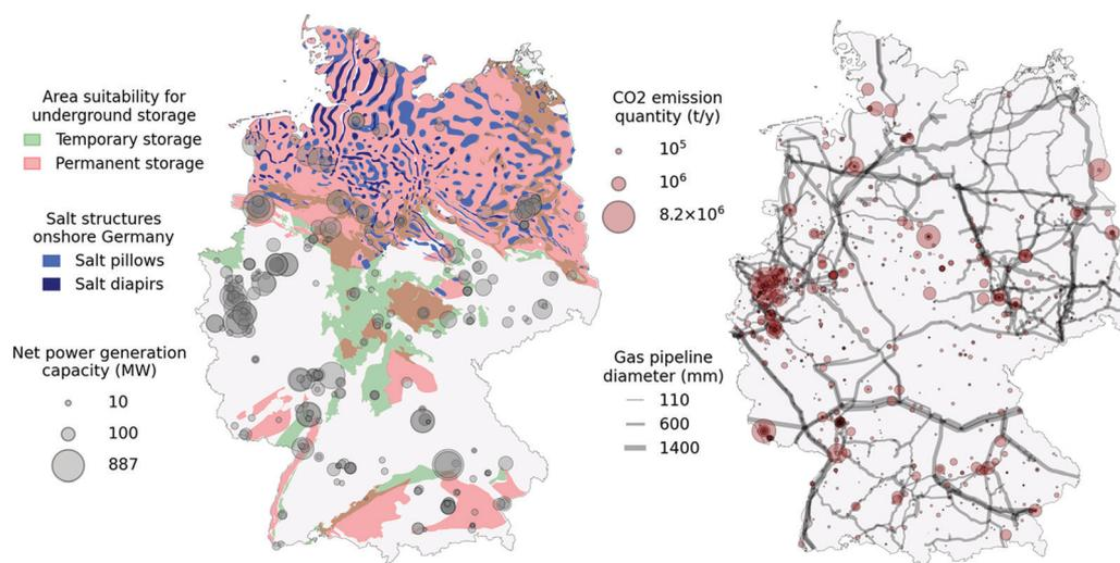
Fig. 4 Map showing relevant underground storage potential for salt structures and porous rocks. Point sources showing quantities of emitted CO<sub>2</sub> registered within the ETS are shown as grey circles.
