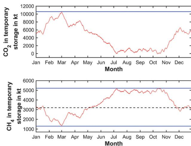
Fig. 12 Cyclical charging and discharging of CO<sub>2</sub> and CH<sub>4</sub> storage on a national scale (the upper blue lines indicate the storage capacities required; the lower blue line indicates the minimum storage quantity of CH<sub>4</sub> and the dashed black line represents the average stored quantity of CH<sub>4</sub> in the subsurface storage based on the chosen initial storage value).
