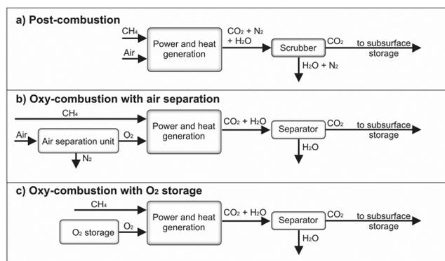
Fig. 3 Process routes for heat and power generation including CO<sub>2</sub> separation.
