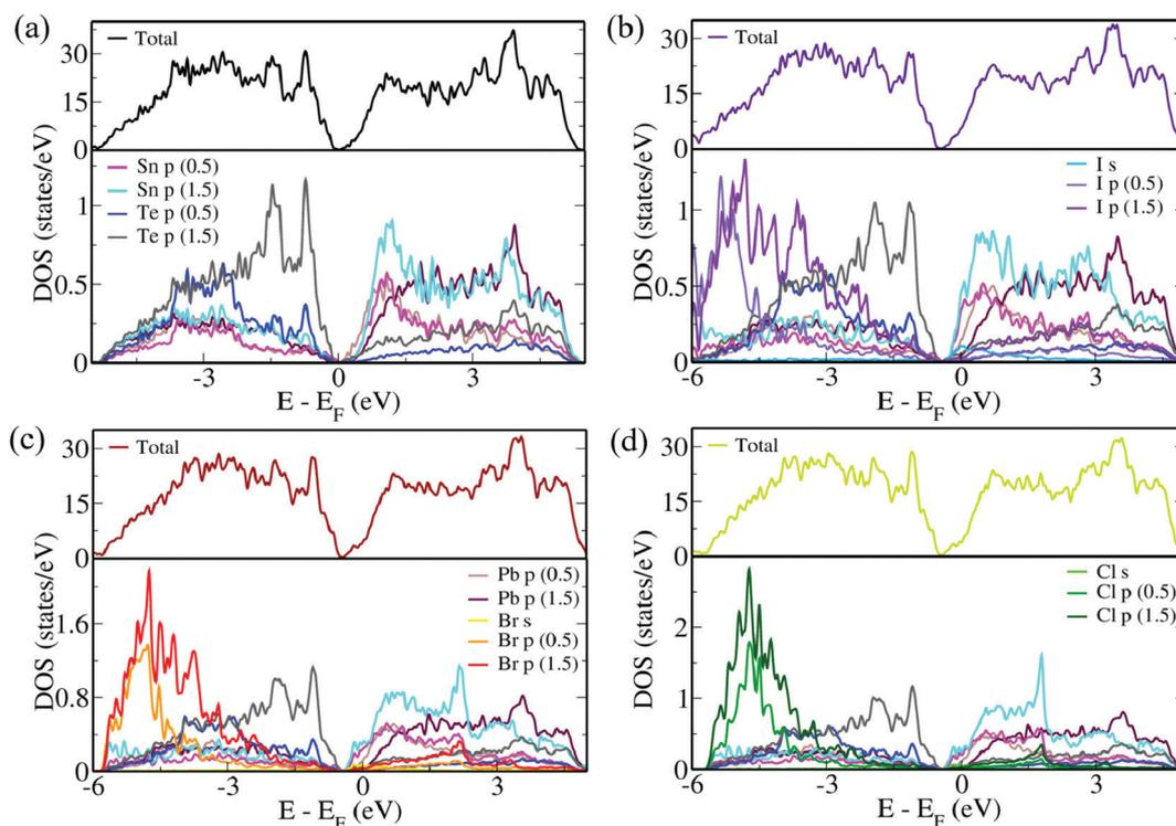
Fig. 2 pDOS of (a)  $\text{Pb}_{10}\text{Sn}_6\text{Te}_{16}$ , (b)  $\text{Pb}_{10}\text{Sn}_6\text{Te}_{15}\text{I}$ , (c)  $\text{Pb}_{10}\text{Sn}_6\text{Te}_{15}\text{Br}$  and (d)  $\text{Pb}_{10}\text{Sn}_6\text{Te}_{15}\text{Cl}$ . Energy is shifted with respect to the Fermi level, which is set to zero.
