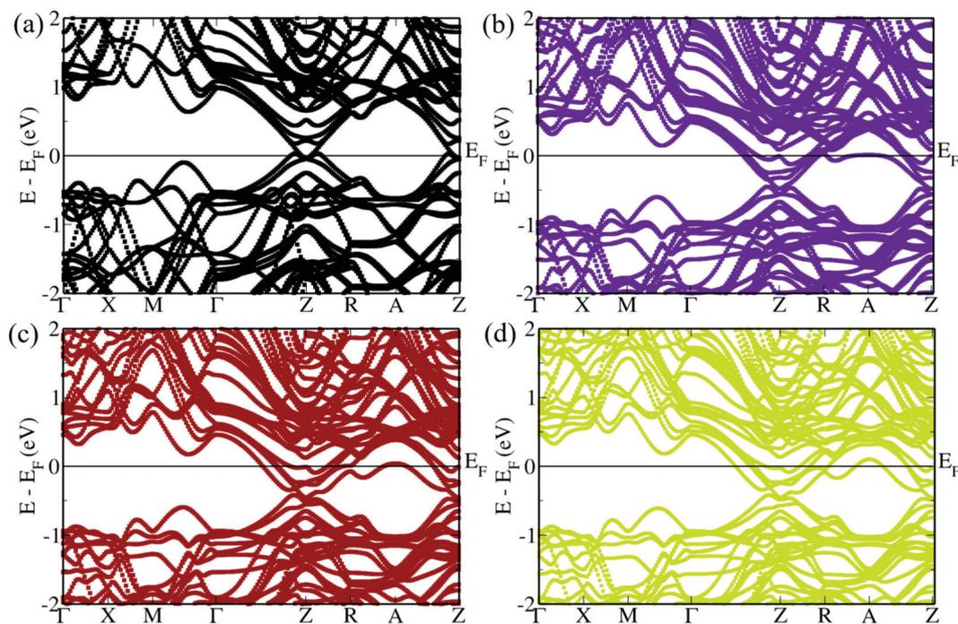
Fig. 1 Electronic structure of (a)  $\text{Pb}_{10}\text{Sn}_6\text{Te}_{16}$ , (b)  $\text{Pb}_{10}\text{Sn}_6\text{Te}_{15}\text{I}$ , (c)  $\text{Pb}_{10}\text{Sn}_6\text{Te}_{15}\text{Br}$  and (d)  $\text{Pb}_{10}\text{Sn}_6\text{Te}_{15}\text{Cl}$ . Energy is shifted with respect to the Fermi level, which is set to zero.
