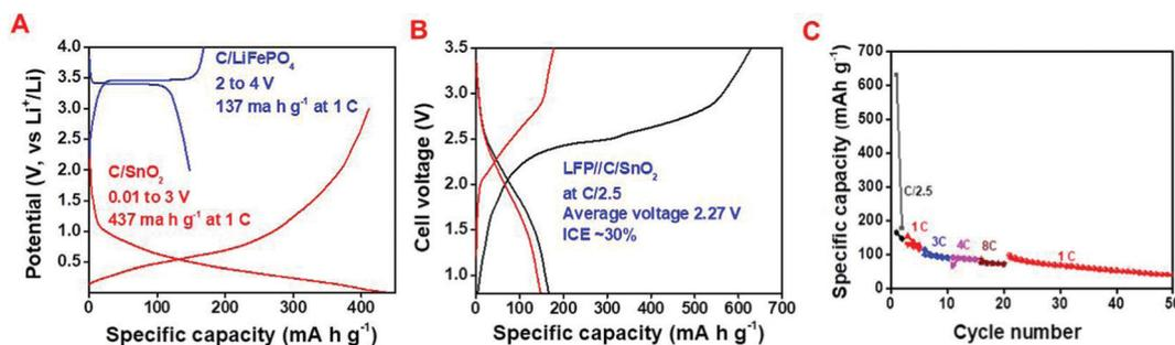
Fig. 6 Full cell analysis; C/LFP as the cathode and C/SnO<sub>2</sub> as the anode; (A) charge–discharge profile of C/LFP and C/SnO<sub>2</sub> at 1C in the half cell, (B) charge–discharge curve at C/2.5 and (C) rate capability curve of the full cell.
