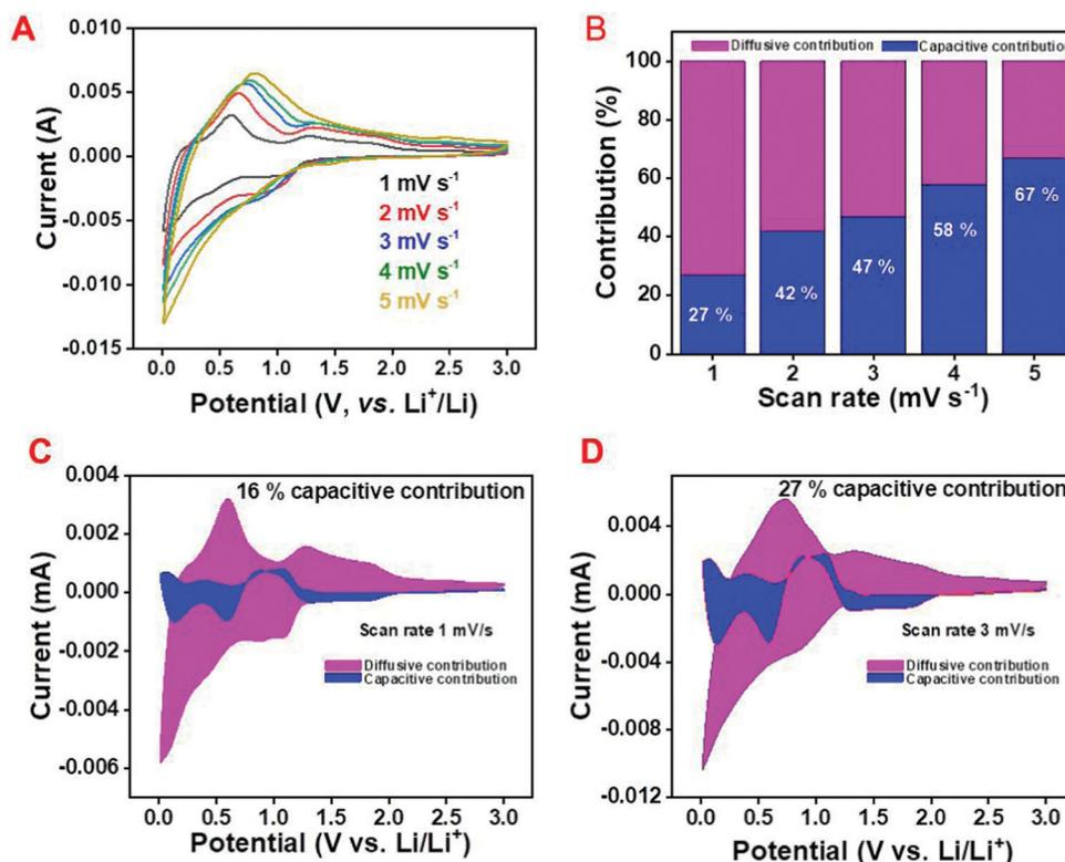
Fig. 4 Kinetics of the Li-ion in the  $\text{C/SnO}_2$  composite; (A) cyclic voltammogram, (B) capacitive and diffusive contribution curve at different scan rates for a fixed potential (at  $0.58 \text{ V}$ ), and capacitive and diffusive contribution in a cyclic voltammogram for a fixed scan rate, (C)  $1 \text{ mV s}^{-1}$  and (D)  $3 \text{ mV s}^{-1}$ .
