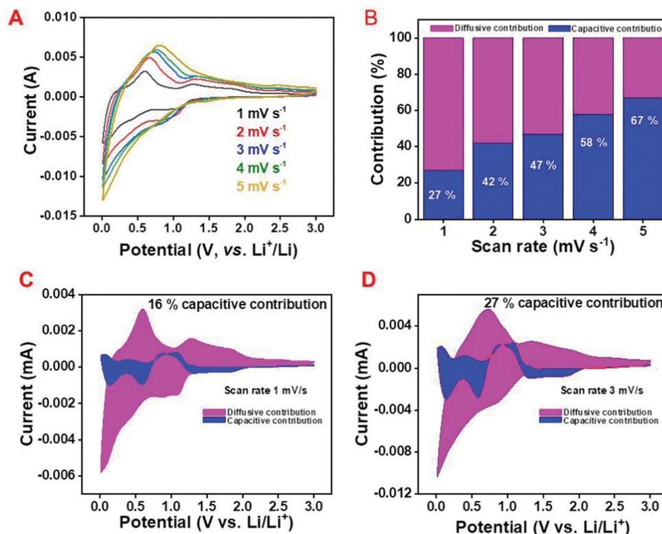
Fig. 4 Kinetics of the Li-ion in the  $\text{C}/\text{SnO}_2$  composite; (A) cyclic voltammogram, (B) capacitive and diffusive contribution curve at different scan rates for a fixed potential (at  $0.58 \text{ V}$ ), and capacitive and diffusive contribution in a cyclic voltammogram for a fixed scan rate, (C)  $1 \text{ mV s}^{-1}$  and (D)  $3 \text{ mV s}^{-1}$ .
