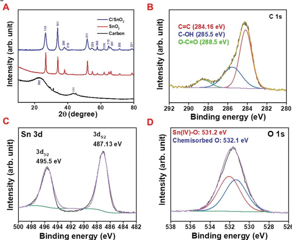
Fig. 2 (A) Comparative X-ray diffraction pattern of NAC (black line), bare SnO<sub>2</sub> (red line) and C/SnO<sub>2</sub> (blue line), X-ray photo electron spectroscopy of the C/SnO<sub>2</sub> composite; (B) C 1s, (C) Sn 3d and (D) O 1s.
