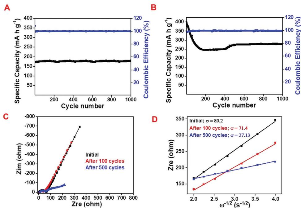
Fig. 5 Cyclic stability curve for (A) NAC at  $200 \text{ mA g}^{-1}$  and (B) C/SnO<sub>2</sub> at  $375 \text{ mA h g}^{-1}$ , (C) electrochemical impedance spectra (EIS) of C/SnO<sub>2</sub> at different stages of the cycles, (D) real impedance ( $Z_{re}$ ) vs. angular frequency ( $\omega$ ) plot where the slope refers to the Warburg impedance coefficient ( $\sigma$ ).
