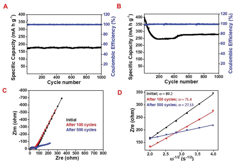
Fig. 5 Cyclic stability curve for (A) NAC at  $200 \text{ mA g}^{-1}$  and (B) C/SnO<sub>2</sub> at  $375 \text{ mA h g}^{-1}$ , (C) electrochemical impedance spectra (EIS) of C/SnO<sub>2</sub> at different stages of the cycles, (D) real impedance ( $Z_{re}$ ) vs. angular frequency ( $\omega$ ) plot where the slot refers to the Warburg impedance coefficient ( $\sigma$ ).
