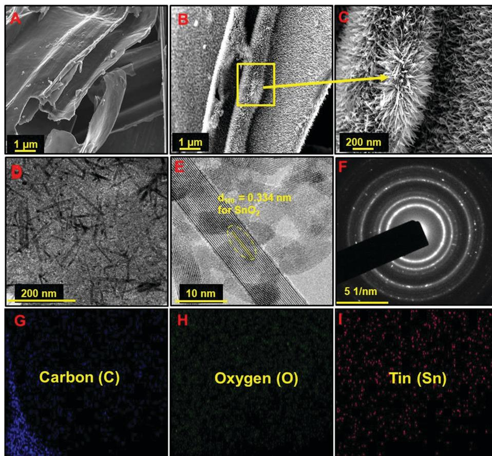
Fig. 1 FESEM images of (A) non-activated carbon (NAC) and (B and C) C/SnO<sub>2</sub>, (D) TEM image, (E) HRTEM image and (F) SAED pattern of C/SnO<sub>2</sub>. (F–I) Elemental area mapping of the C/SnO<sub>2</sub> composite from the TEM image.
