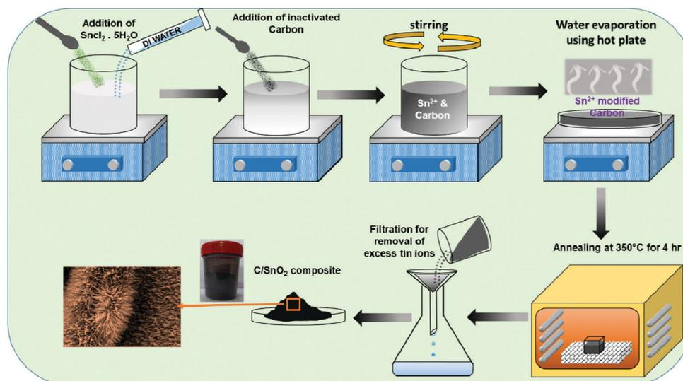
Scheme 1 Schematic presentation of the synthesis of the C/SnO<sub>2</sub> composite using the chemical dispersion method followed by annealing technique.
