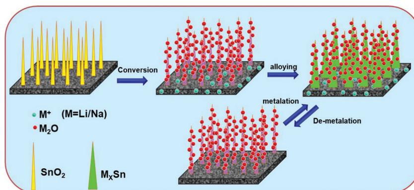
Scheme 2 Schematic presentation of the Li/Na-ion insertion and de-insertion reaction mechanism of the C/SnO<sub>2</sub> composite.
