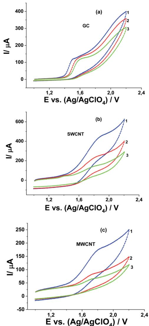
Fig. 8 CVs of 1.0 mM Pyr<sub>1</sub> and 0.5 M MeOH in 0.1 M Bu<sub>4</sub>NClO<sub>4</sub> solution in MeCN in the presence of CH<sub>3</sub>COOH: (1) 0, (2) 1.0, and (3) 2.0 M at (a) (GC), (b) SWCNT and (c) MWCNT paper electrodes at a potential scan rate of 50 mV s<sup>-1</sup>.
