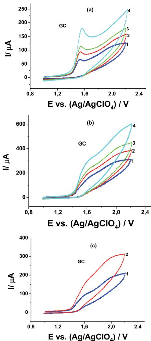
Fig. 3 CVs of 0.1 M  $\text{Bu}_4\text{NClO}_4$  solution in MeCN at the GC electrode in the presence of: (a) 1 mM  $\text{Pyr}_1$  and 0.01 M MeOH at potential scan rates of: (1) 20, (2) 50, (3) 80, and (4) 200  $\text{mV s}^{-1}$ ; (b) 1 mM  $\text{Pyr}_1$  and 0.5 M MeOH at potential scan rates of: (1) 20, (2) 50, (3) 80, and (4) 200  $\text{mV s}^{-1}$ ; and (c) 0.5 M MeOH and  $\text{Pyr}_1$ : (1) 0.5 mM and (2) 1 mM at a potential scan rate of 20  $\text{mV s}^{-1}$ .
