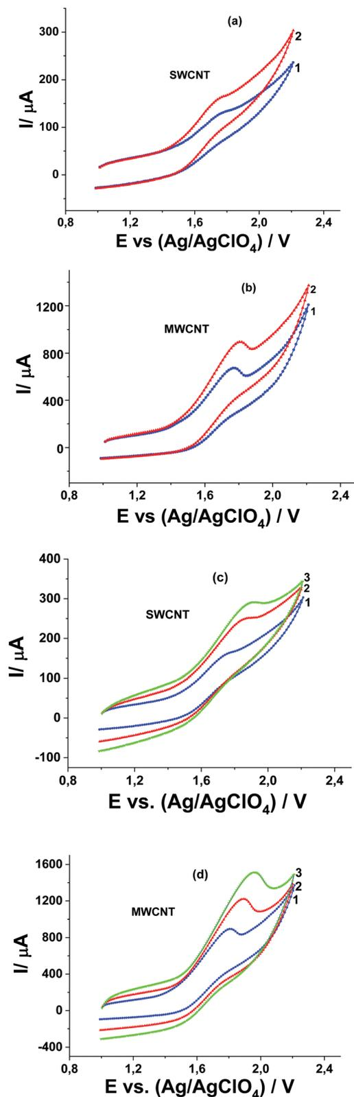
Fig. 6 CVs of 0.1 M  $\text{Bu}_4\text{NClO}_4$  solution in MeCN in the presence of 0.5 M MeOH and  $\text{Pyr}_1$ : (1) 0.5 mM and (2) 1 mM at a potential scan rate of  $20 \text{ mV s}^{-1}$  at (a) SWCNT and (b) MWCNT paper electrodes and in the presence of 1 mM  $\text{Pyr}_1$  and 0.5 M MeOH at potential scan rates of: (1) 20, (2) 50, and (3)  $80 \text{ mV s}^{-1}$  at (c) SWCNT and (d) MWCNT paper electrodes.
