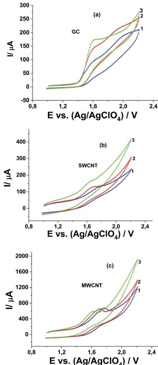
Fig. 9 CVs of 0.5 mM Pyr<sub>1</sub> and 0.5 M MeOH in 0.1 M Bu<sub>4</sub>NClO<sub>4</sub> solution in MeCN in the presence of H<sub>2</sub>O: (1) 0, (2) 0.5, and (3) 2.0 M at (a) (GC), (b) SWCNT and (c) MWCNT paper electrodes at a potential scan rate of 20 mV s<sup>-1</sup>.
