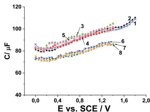
Fig. 7 Dependences of the differential capacitance  $C$  of the MWCNT paper electrode at a potential  $E$  of 0.1 M  $\text{Bu}_4\text{ClO}_4$  solution in MeCN in the presence of  $\text{Pyr}_1$ : 0 (curves 1 and 2) and 1 mM (curves 3–5), 1 mM  $\text{Pyr}_1$  and 0.5 M MeOH (curve 6–8). Curves 1 and 2 were recorded just after recording the cyclic voltammograms, and curves 3, 4 and 5 are settled curves.
