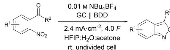
+ galvanostatic mode + undivided cell + scalable
