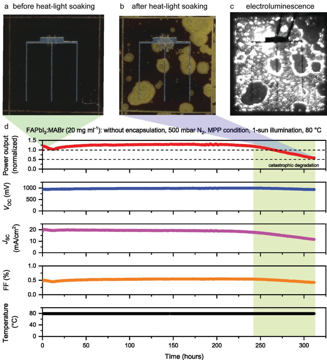
Fig. 7 Operational stability of FAPbI<sub>3</sub>:MABr (20 mg ml<sup>-1</sup>) solar cells. (a and b) Photographs of the cell before (a) and after (b) 320 hours MPP operation at 80 °C under a 500 mbar N<sub>2</sub> atmosphere. (c) The corresponding electroluminescence (EL) image of the same cell. (d) The photovoltaic parameters of the cell during 320 hours MPP operation at 80 °C under a 500 mbar N<sub>2</sub> atmosphere.
