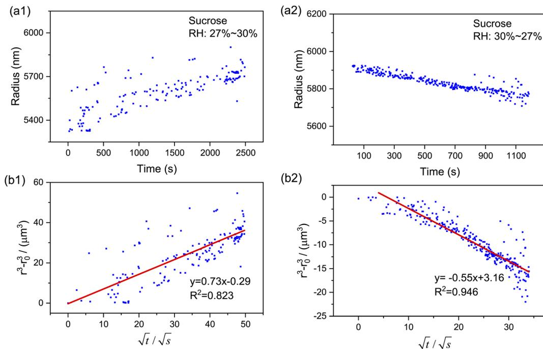
Fig. 4 Size-response of the sucrose droplets to RH changes. Time evolution of the radius when RH changed from 27% to 30% (a1) and from 30% to 27% (a2), respectively. Relationship of  $r^3 - r_0^3$  and  $\sqrt{t}$  when RH changed from 27% to 30% (b1) and from 30% to 27% (b2), respectively. Linear regressions are plotted in red lines.
