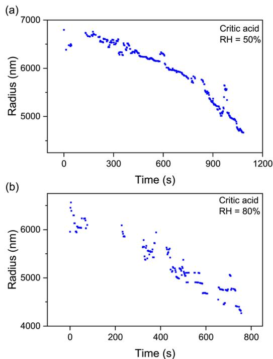
Fig. 5 Time evolution of the radius of droplets of citric acid at constant RH values: (a) RH = 50%; (b) RH = 80%. The sustained decrease of the radius indicates the volatility of CA.
