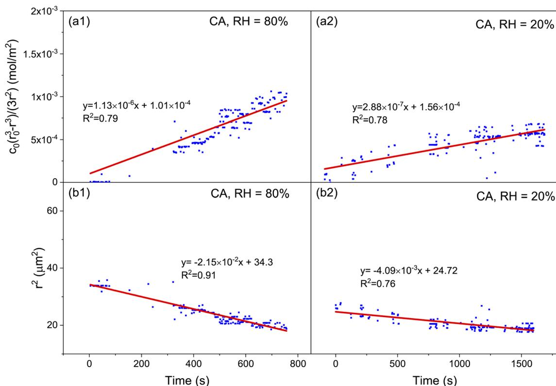
Fig. 6 The volatility of citric acid droplets at constant RH values. Relationship of  $(r_0^3 - r^3)c_0/3r^2$  and  $t$  at RH = 80% (a1) and 20% (a2), which is used to measure the volatile flux. Relationship of  $r^2$  and  $t$  at RH = 80% (b1) and 20% (b2), which is used to measure the vapor pressure. Linear regressions are plotted in red lines.
