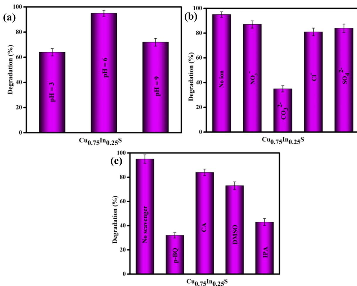
Fig. 5 Degradation efficiency of GMF over 10 ppm  $\text{Cu}_{0.75}\text{In}_{0.25}\text{S}$  photocatalyst on different (a) pH solutions, (b) anions, and (c) scavengers.
