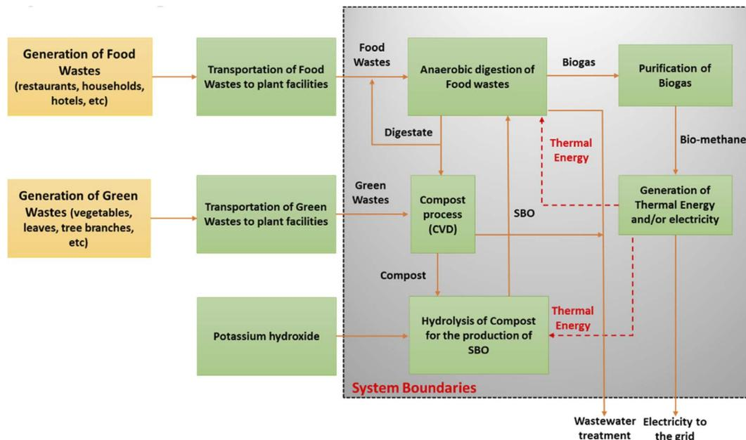
Fig. 1 Scheme of integrated chemical and biochemical processes. Legends: compost of food wastes' digestate and green waste mixture (CVD); soluble biobased product (SBO).
