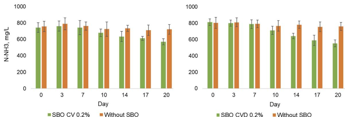
**Fig. 5** Ammonia concentration in the presence and absence of 0.2% CV or CVD SBO during the trials of OT.
