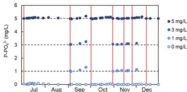
Fig. 4 Stability of the calibration of the PHOSPO-H 4200 automated analyzer in the range 0–5 mg L<sup>-1</sup> of P from July to December, 2019.
