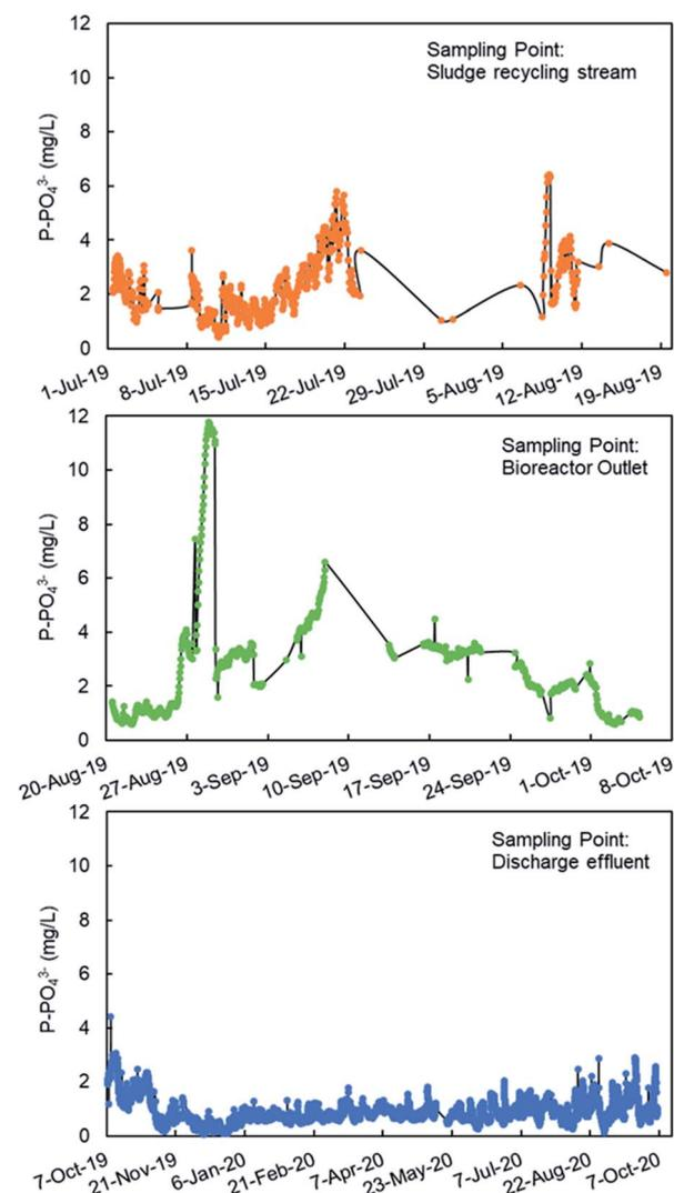
Fig. 6 Phosphate analysis with PHOSPO-H 4200 in three sampling points in the WWTP of Nigrán from July 2019 to October 2020.
