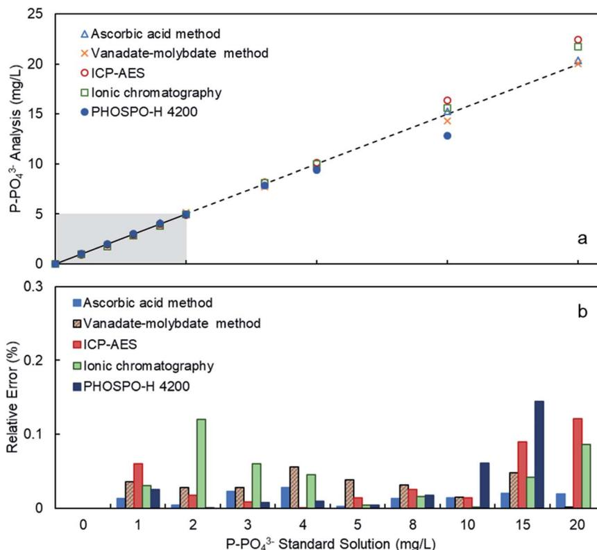
Fig. 3 Calibration of the PHOSPO-H 4200 with phosphate standard solutions in the range 0–5 mg L<sup>-1</sup>. (a) Comparison of the response of the automated analyzer with the four different analytical methods in the University of Vigo. (b) Relative error of the phosphate analysis.
