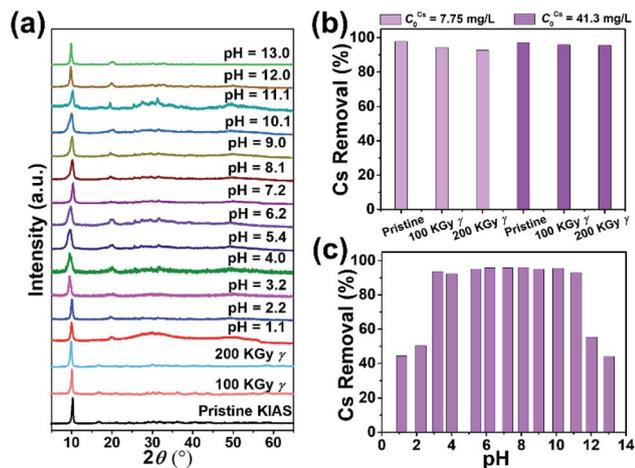
Fig. 4 (a) PXRD patterns of pristine KIAS and the corresponding irradiated samples and  $Cs^{+}$ -exchanged products at different pH values. (b)  $R^{Cs}$  (%) of pristine KIAS and irradiated samples. (c)  $R^{Cs}$  (%) of KIAS at various pH values.
