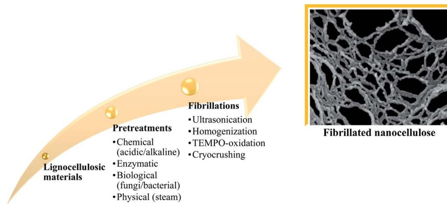
Fig. 7 Nanocellulose isolation stages and types of treatments.<sup>65–69</sup>
