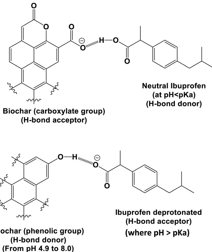
Scheme 4 WSBC hydrogen bonding from ibuprofen (pH < pK<sub>a</sub>) and to ibuprofen (pH > pK<sub>a</sub>).
