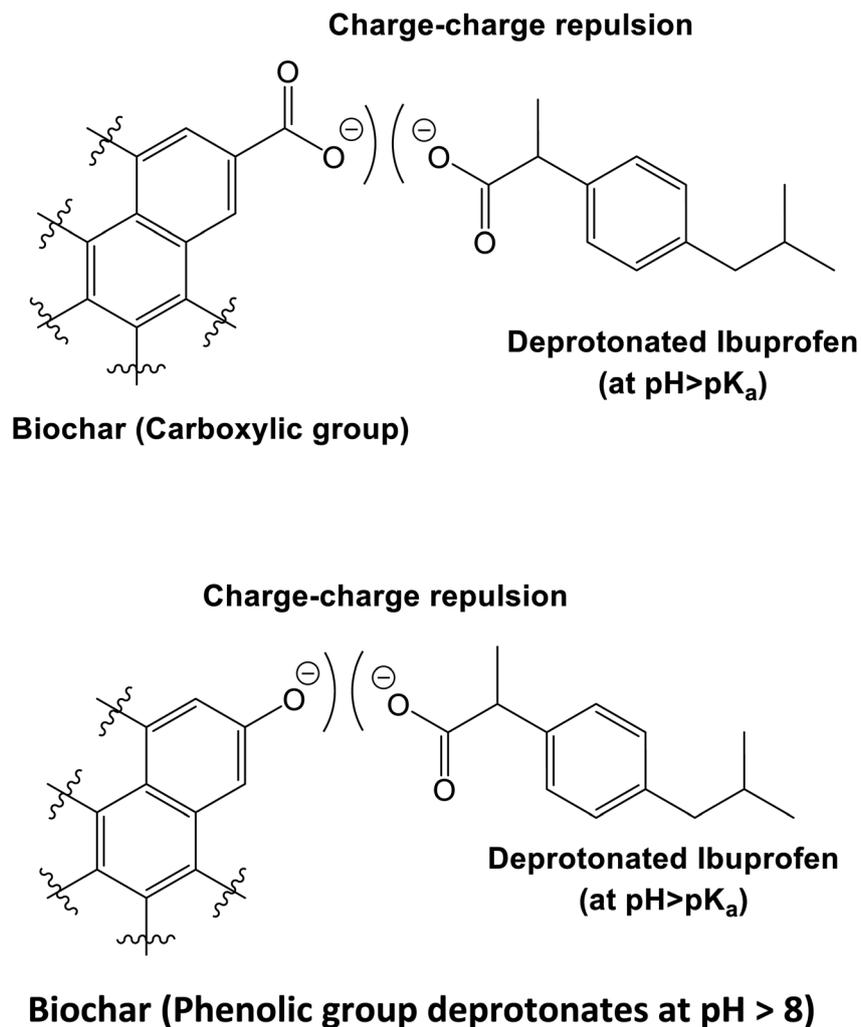
**Scheme 5** At high pH ( $\text{pH} > \text{both } \text{pH}_{\text{zpc}} \text{ and } \text{pK}_a$ ), both ibuprofen and WSAB are negatively charged, leading to charge–charge repulsions, thus decreasing the overall adsorption.
