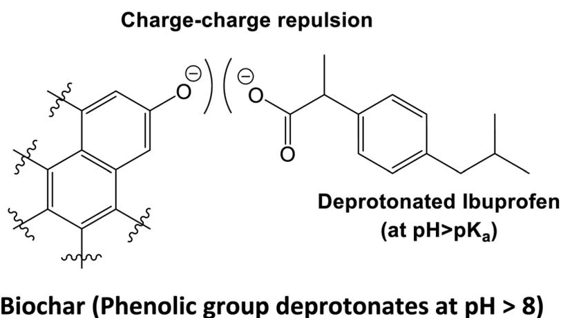
**Scheme 5** At high pH ( $\text{pH} > \text{both } \text{pH}_{\text{zpc}} \text{ and } \text{pK}_{\text{a}}$ ), both ibuprofen and WSAB are negatively charged, leading to charge–charge repulsions, thus decreasing the overall adsorption.
