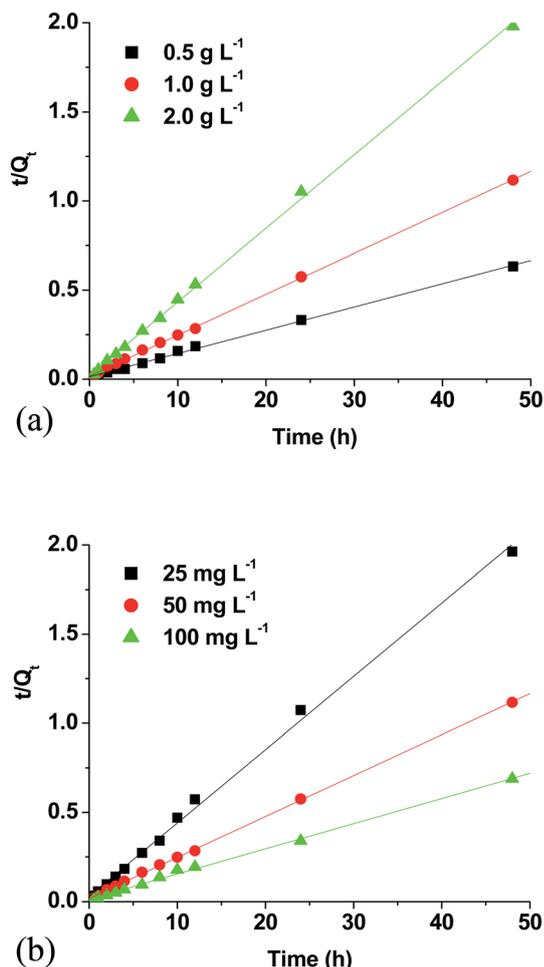
Fig. 3 Pseudo-second order kinetic plots (a) dose kinetics at 0.5, 1.0 and 2.0 g L<sup>-1</sup> WSAB; (b) ibuprofen conc. kinetics at 25, 50, and 100 mg L<sup>-1</sup> [temp. 25 °C, pH 4.0].
