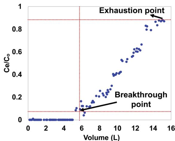
Fig. 6 Ibuprofen uptake on WSAB fixed-bed column. A graph showing the breakpoint and saturation at the exhaustion point (initial ibuprofen concentration 7.5 mg L<sup>-1</sup>, pH 4.0, and column bed length ~4 cm; hydraulic flow rate of 2.5 mL min<sup>-1</sup>; WSAB dose 2.0 g).
