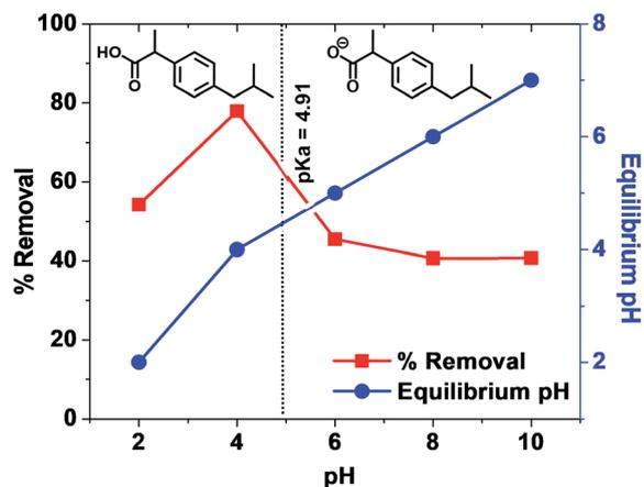
Fig. 5 Effect of the initial pH on ibuprofen sorption using WSAB [temperature 25 °C, initial ibuprofen concentration 50 mg L<sup>-1</sup>, and WSAB dose 1.0 g L<sup>-1</sup>].
