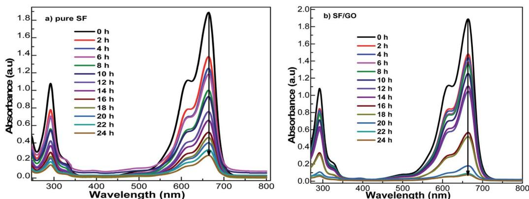
Fig. 6 UV-Vis spectral changes during MB uptake on (a) pristine SF and (b) SF/GO film at different contact times.
