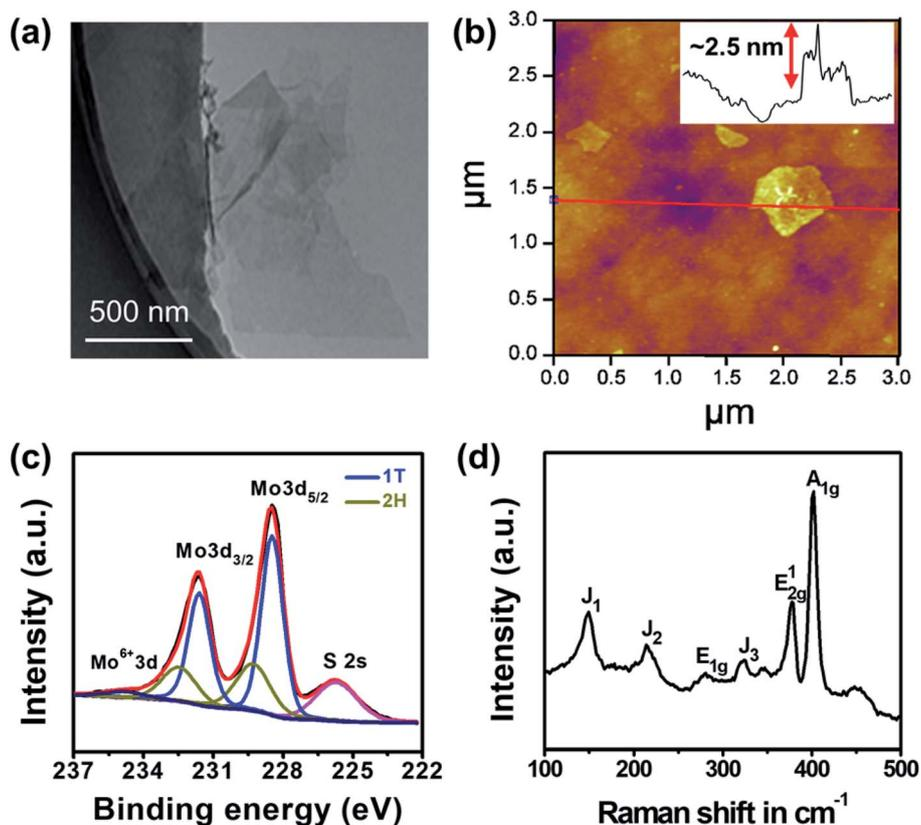
Fig. 1 Characterization of the as-exfoliated MoS<sub>2</sub> nanosheets. (a) TEM and (b) AFM images of MoS<sub>2</sub> nanosheets, and the inset shows the line profile; (c) Mo 3d XPS and (d) Raman spectra.
