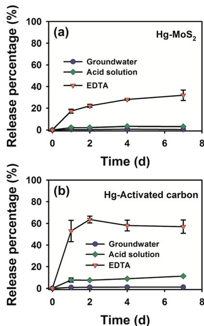
Fig. 5 Desorption kinetics of Hg from (a) MoS<sub>2</sub> and (b) activated carbon in the groundwater, acid solution, and EDTA solution, initial  $C_{\text{Hg}} = 20 \text{ mg L}^{-1}$ ,  $C_{\text{MoS}_2} = 8 \text{ mg L}^{-1}$ ,  $C_{\text{AC}} = 1.67 \text{ g L}^{-1}$ .
