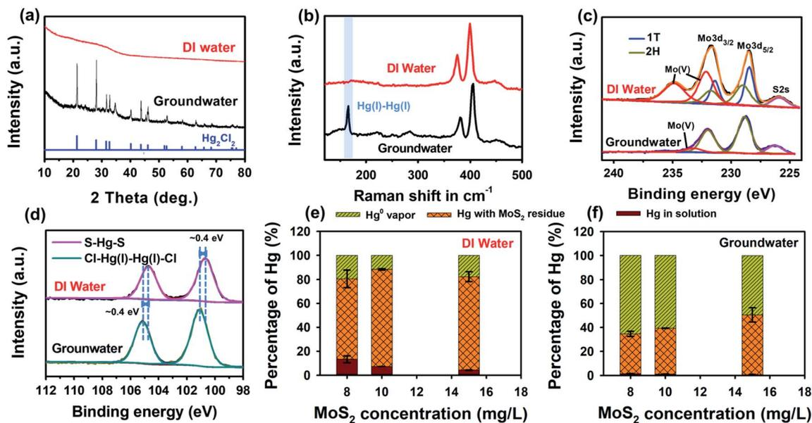
Fig. 3 Mechanistic investigation of Hg(II) removal by MoS<sub>2</sub> nanosheets in groundwater and DI matrices. (a) XRD patterns, (b) Raman spectra, (c) Mo 3d and (d) Hg 4f XPS spectra of Hg-laden MoS<sub>2</sub> formed in DI water and groundwater; Hg species distribution in the Hg-laden MoS<sub>2</sub> nanosheets formed in (e) DI water and (f) groundwater.
