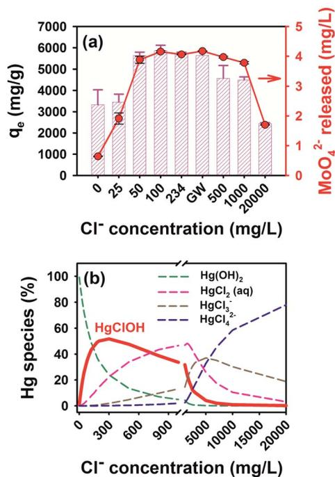
Fig. 4 Speciation-dependent Hg removal efficiency varied by  $\text{Cl}^-$  concentrations. (a) Effects of  $\text{Cl}^-$  on Hg removal by  $\text{MoS}_2$ ,  $C_{\text{Hg}} = 35 \text{ mg L}^{-1}$  and  $C_{\text{MoS}_2} = 4 \text{ mg L}^{-1}$ . (b) Hg speciation as a function of  $\text{Cl}^-$  concentration determined by using Visual MINTEQ.
