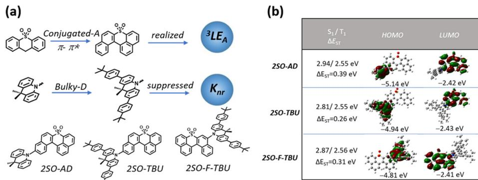
Fig. 1 (a) Schematic diagram of the molecular design strategy; (b) HOMO and LUMO electronic distributions, and the lowest singlet ( $S_1$ ) and triplet ( $T_1$ ) energy levels for 2SO-AD, 2SO-TBU and 2SO-F-TBU calculated by DFT at the B3LYP/6-31g(d,p) level.
