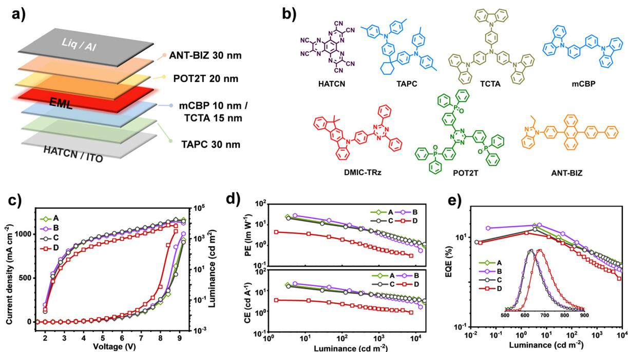
Fig. 5 (a) The diagram of OLED structures, and (b) chemical structures of the used materials. (c) The current density–voltage–luminance ( $J$ – $V$ – $L$ ) curves of these devices. (d) Power efficiency and current efficiency as a function of luminance, and (e) EQE curves versus luminance, and EL spectra (inset, at the same driving voltage of 2.8 V) of these involved devices (A–D).
