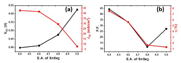
Fig. 5 Effect of electron affinity on the parameters  $V_{oc}$ ,  $J_{sc}$  (a), FF, and efficiency ( $\eta$ ) (b) of the SnSe-based solar device.
