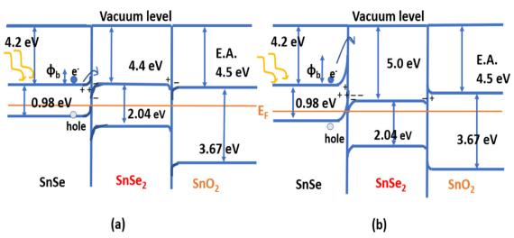
Fig. 6 Schematic diagram of the band alignment of the configuration when the E.A. of SnSe<sub>2</sub> is (a) 4.4 eV and (b) 5.0 eV. E.A. (5.0 eV) makes the barrier a greater height and creates a potential well in the transportation of the carriers.
