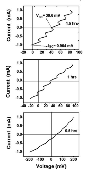
Fig. 4  $\,$   $I\!-\!V$  characteristics of the solar cell devices under AM 1.5G optical power.
